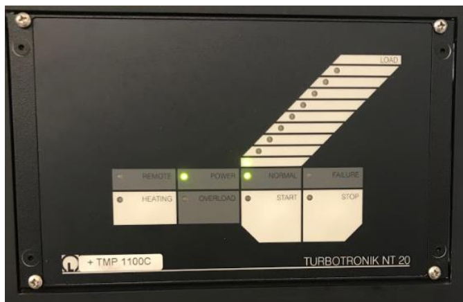
Figure 11: Turbo Pump Control Panel on Blue TVAC
