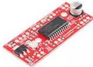
Figure 5-3. Stepper Motor Driver
