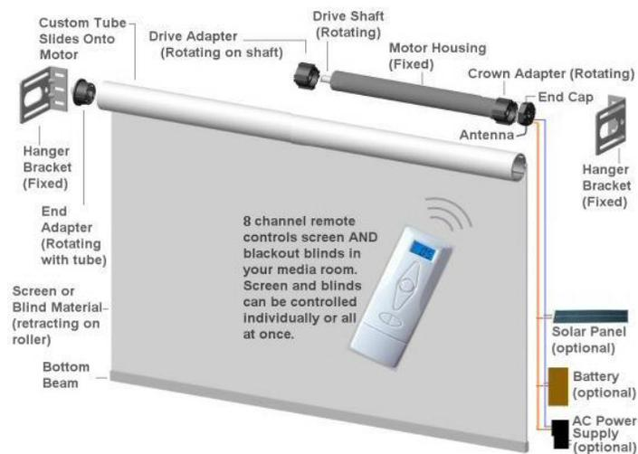
Figure 2-2. Motorized Blinds Controlling a Screen
