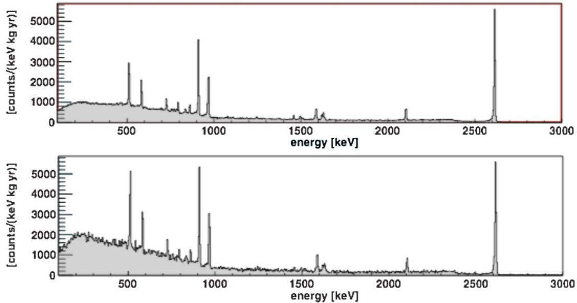
FIG. 3. Typical calibration spectra of the CUORICINO array with a  $^{232}\text{Th}$  source:  $5 \times 5 \times 5 \text{ cm}^3$  crystals upper frame,  $3 \times 3 \times 6 \text{ cm}^3$  crystals lower frame.
