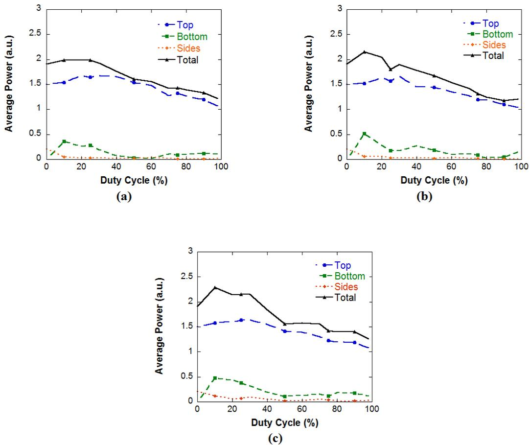
*Figure 7: Output power for grating width: (a) 125nm, (b) 230nm, (c) 460nm with an ITO layer thickness of 78nm*
