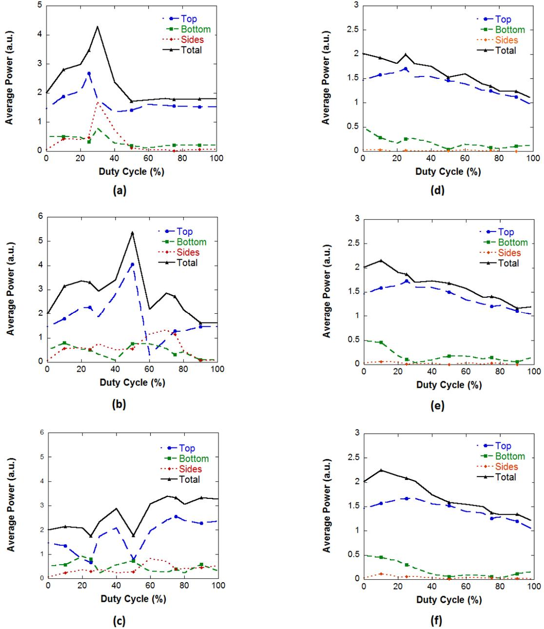
Figure 10: Output power for triangular (a-c) and square (d-e) gratings for grating width: (a,d) 125nm, (b,e) 230nm and (c,f) 460nm with an ITO layer thickness of 230nm
