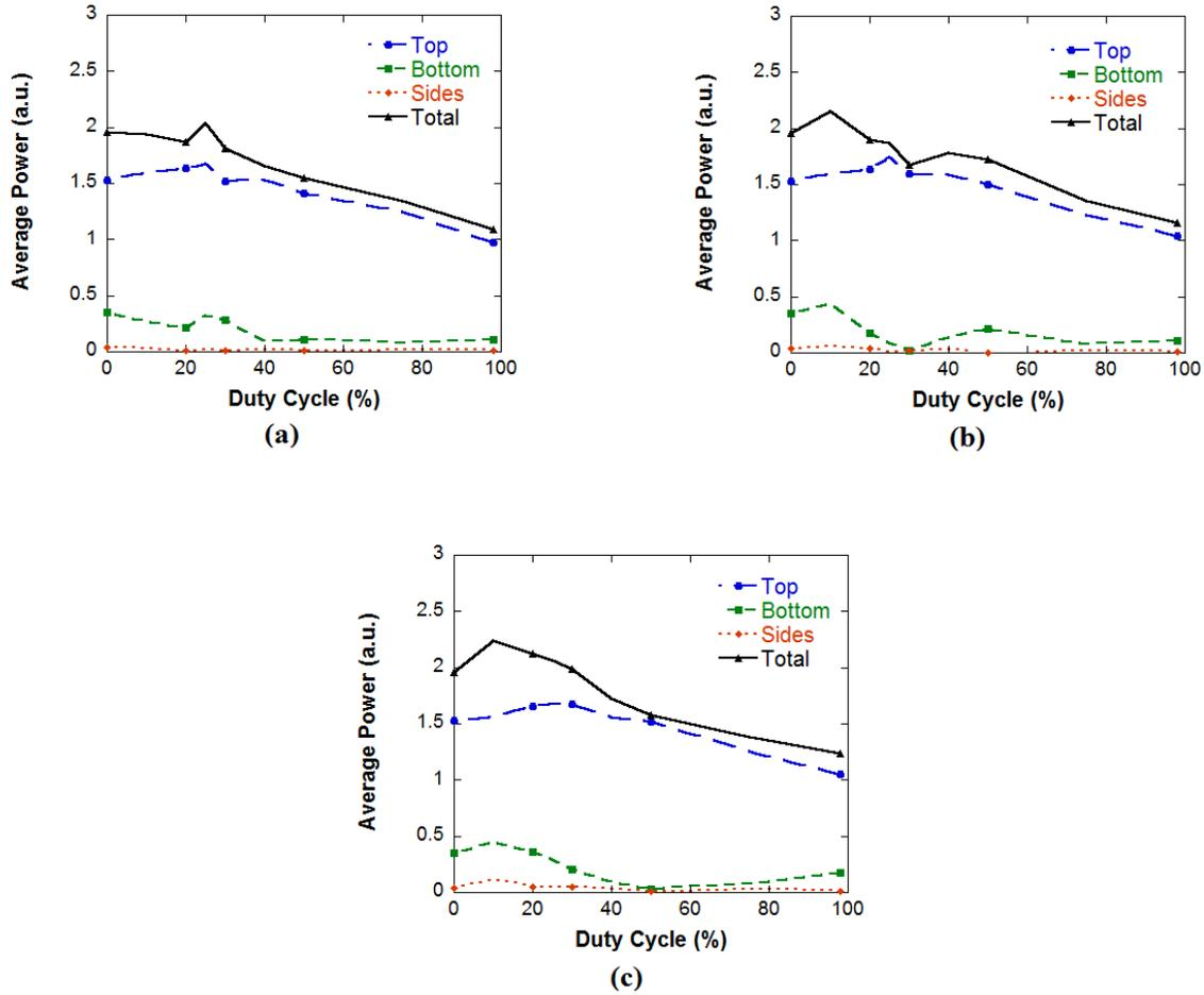
*Figure 9: Output power for grating width: (a) 125nm, (b) 230nm, (c) 460nm with an ITO layer thickness of 260nm*
