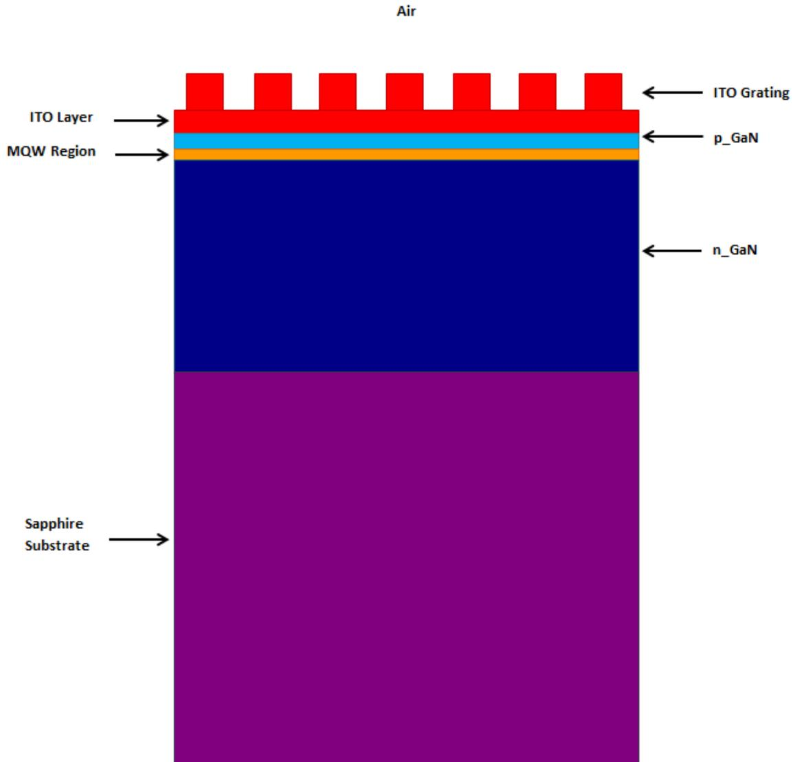
*Figure 5: ITO based grating LED simulation model*
