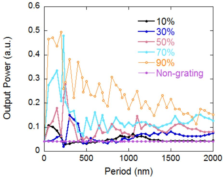
*Figure 2: Output power extracted plotted against grating period at a location of 150nm*
