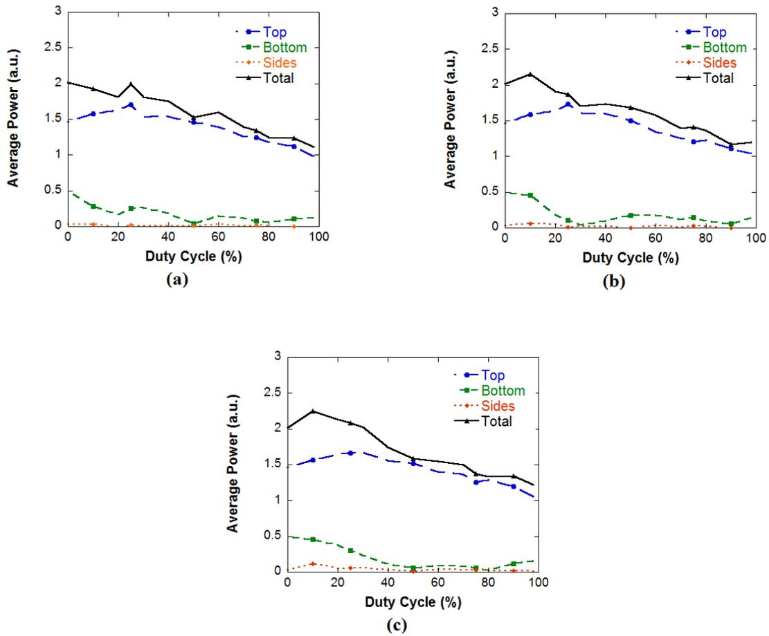
*Figure 8: Output power for grating width: (a) 125nm, (b) 230nm, (c) 460nm with an ITO layer thickness of 230nm*
