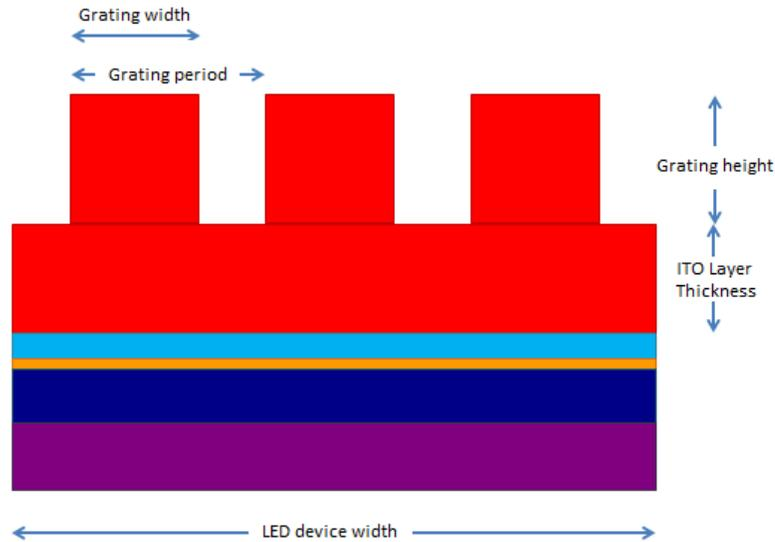
*Figure 6: Transmission grating GaN LED model*
