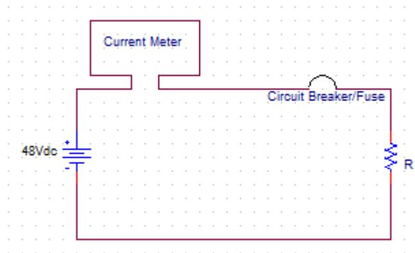
Figure 4-1: Testing Set-Up for Circuit Breaker and Fuse
