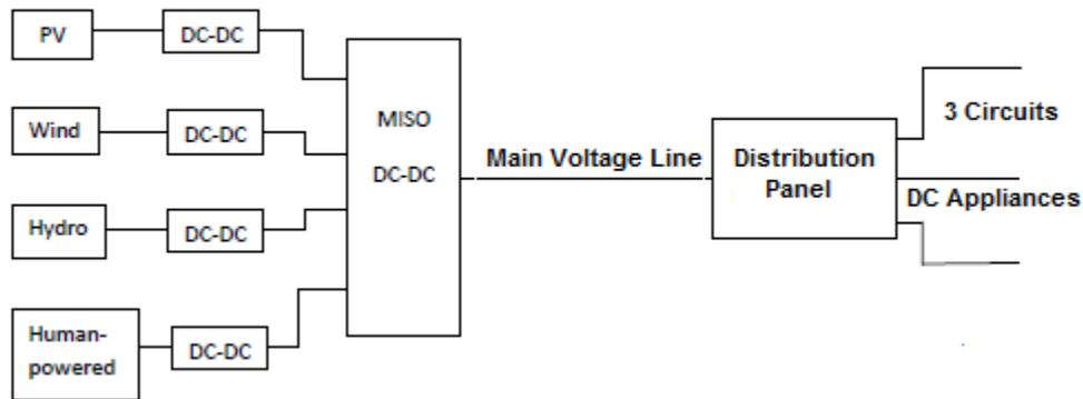
Figure 2-1: System Block Diagram of DC House
