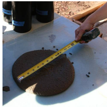
FIG. 2. Testing for Flow
