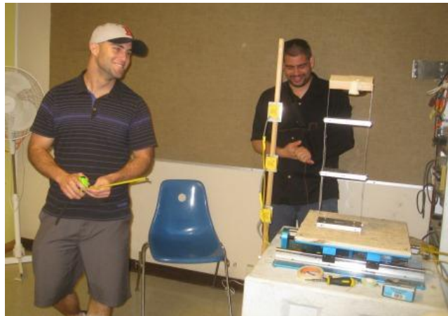
Master's students Adam Rendon and Ken Singh demonstrate building mode shapes on the mini-shake table
