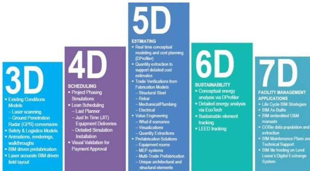
Figure 2 - Dimensions of BIM (Autodesk Revit, 2017)
