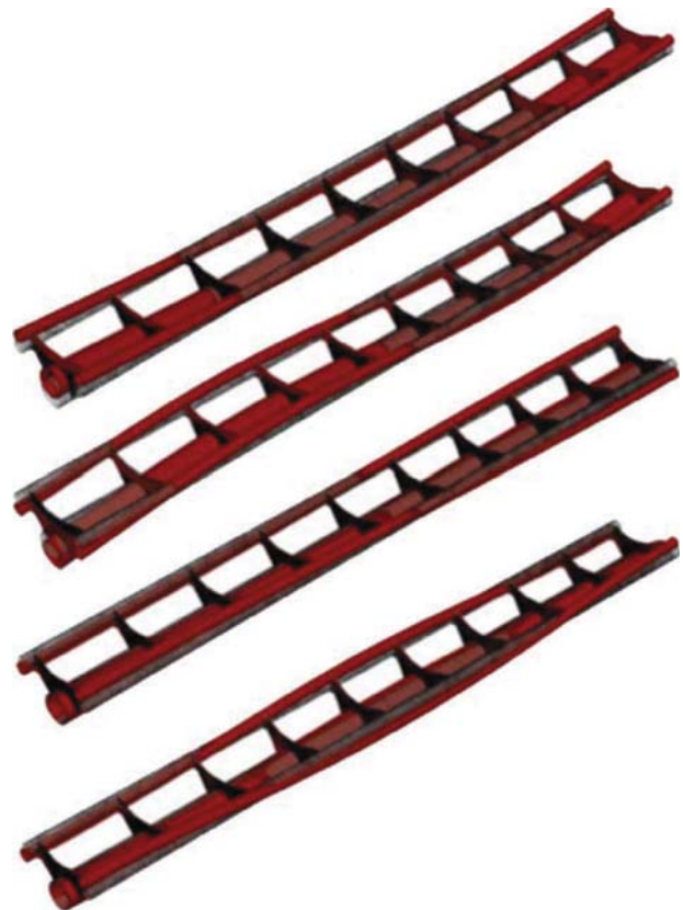
Fig. 5—Bending and torsion modes: top 1st bending mode (19 Hz), 2nd from top second bending mode (49 Hz), 3rd: first torsion mode (20 Hz), 4th: second torsion mode (46 Hz).
