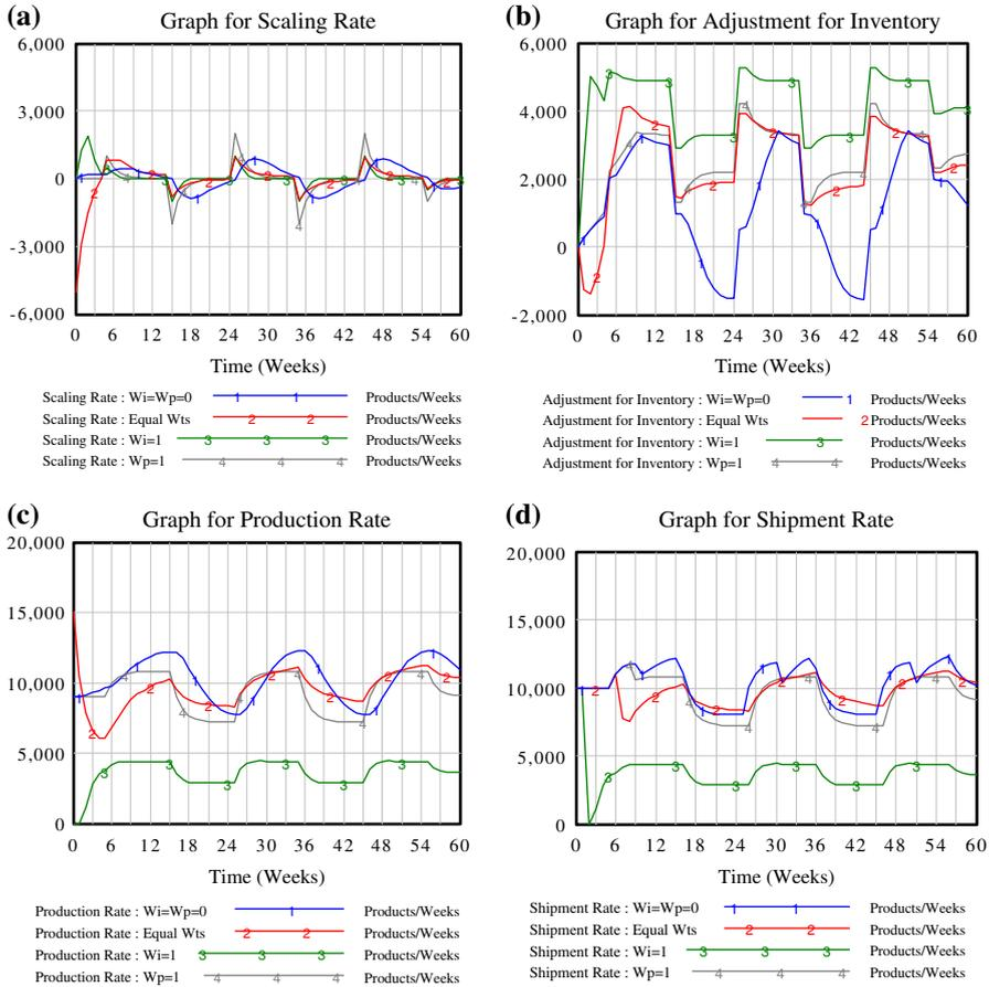
**Fig. 7** Dynamic response for different rates in the developed RMS capacity scalability model in a sudden demand scenario. **(a)** Capacity Scaling Rate, **(b)** Inventory Adjustment Rate, **(c)** Production Rate, **(d)** Shipment Rate
