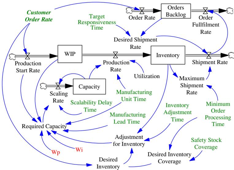
**Fig. 1** Model structure for capacity scalability in RMS
