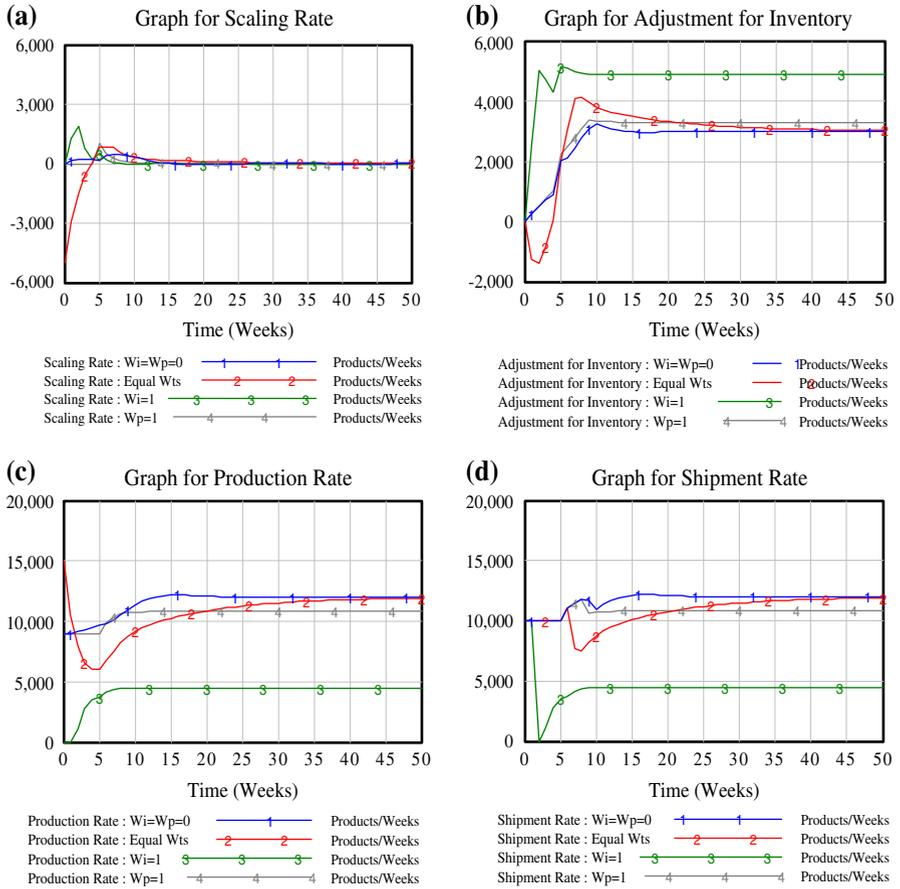
**Fig. 4** Dynamic response for different rates in the developed RMS capacity scalability model in a sudden demand scenario. (a) Capacity Scaling Rate, (b) Inventory Adjustment Rate, (c) Production Rate, (d) Shipment Rate
