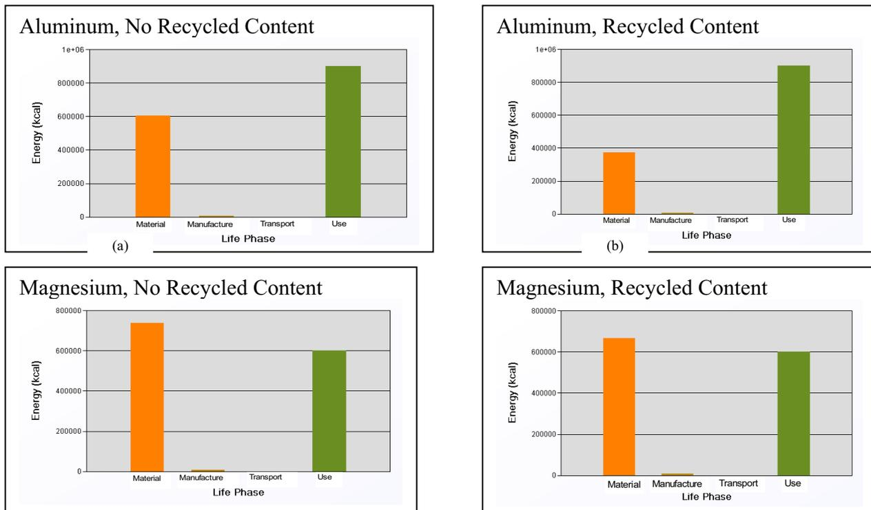
Figure 5. Energy consumption over life of top two materials
