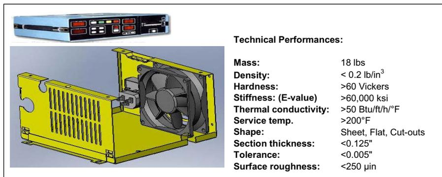
Figure 3. Technical data for the casing of a medical diagnostic equipment
