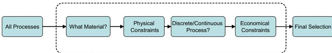
Figure 2. Process selection stages
