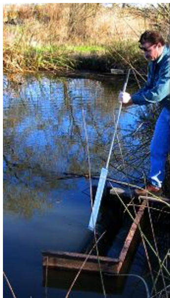
Figure 1. Using the ITRC weir stick to clear weeds in front of a weir.
