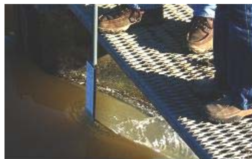
Figure 2. Front view of ITRC Weir Stick being placed on the top of a check for a flow rate measurement.
