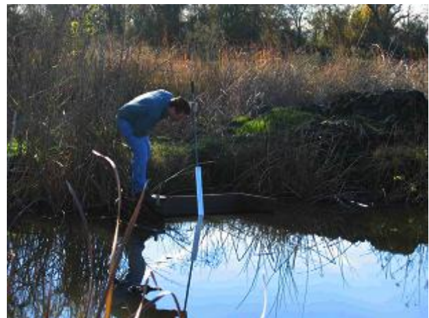
Figure 4. Reading a small flow rate using the ITRC Weir Stick on a spill site
