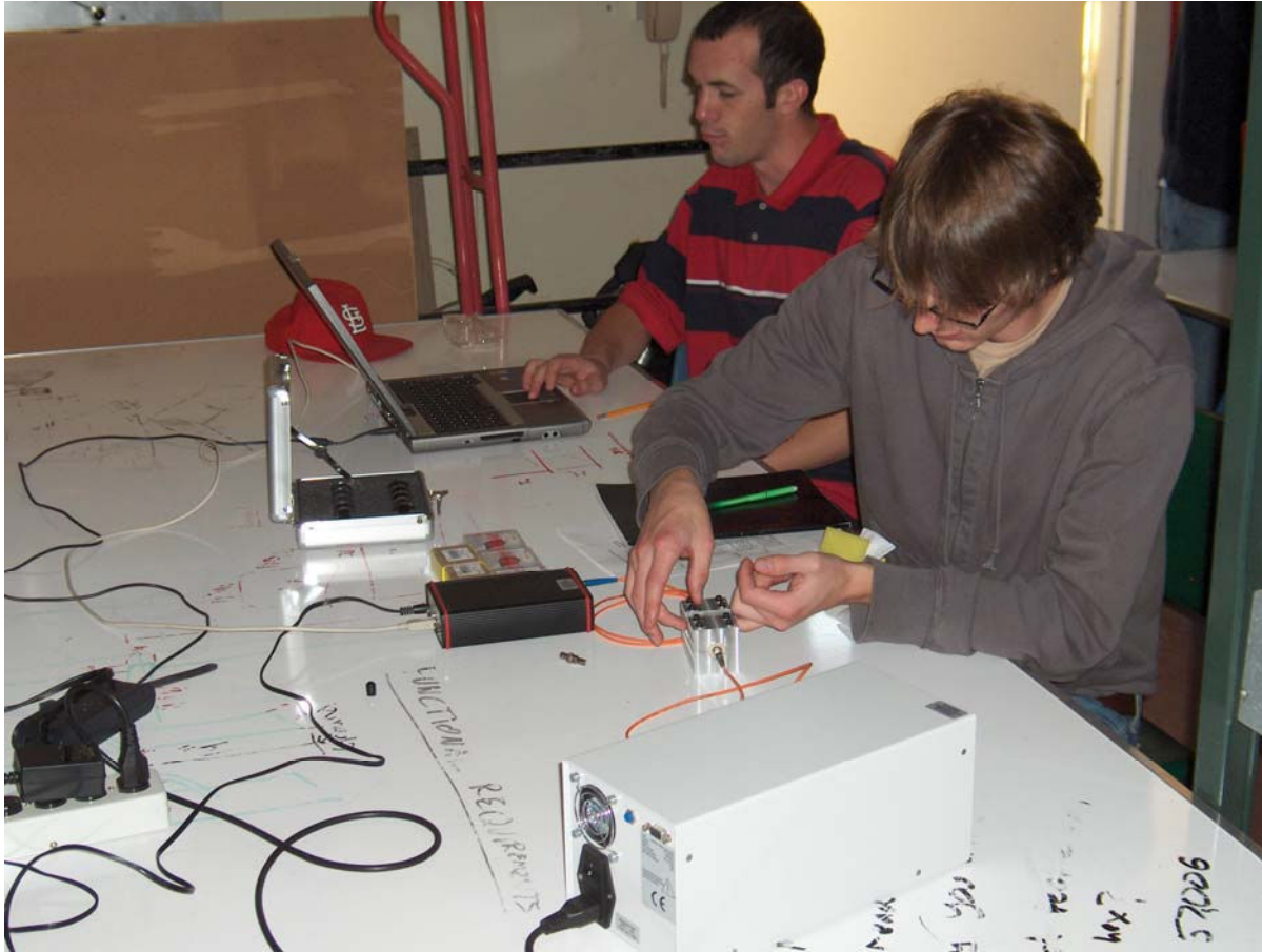
Figure 2 – Students characterizing optical filters with light measurement system they built
