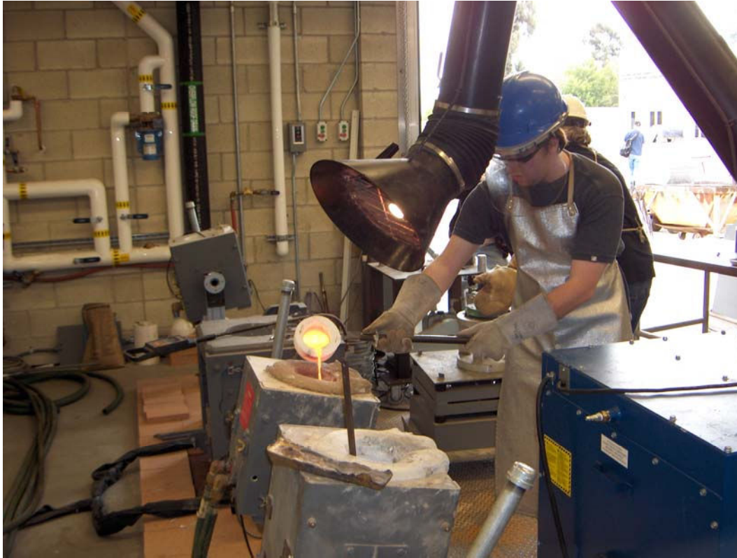
Figure 2 – Pouring of metal casting by students
