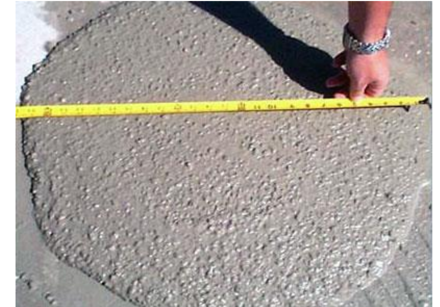
Slump Flow Test (Self-Consolidating Concrete)
