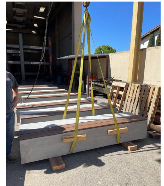
Getting hoist set for the first bench to deliver
