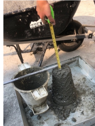
Figure 1: Slump test for Control batch
