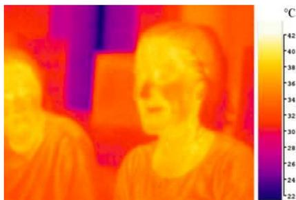
Infrared is used in night-vision equipment when there is insufficient visible light to see an object. The radiation is detected and turned into an image on a screen, hotter objects showing up in different shades than
