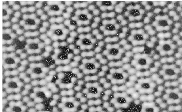
Figure 4: The structure of a silicon crystal imaged with an STM. The empty spaces in the structure are impurities. [8]
