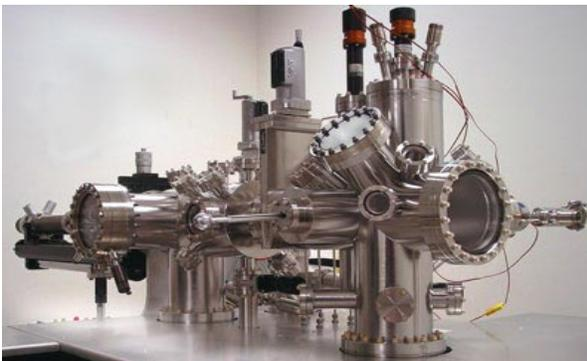
Figure 5: IBM's scanning tunneling microscope. The actual device is inside the large vacuum chamber shown in this image. [9]
