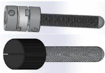
Figure 9: Screws used for adjustment system. The top screw has a coupler for connection to the stepper motor. These screws lower the sample to the tip. Designed by Justin Jee using SOLIDWORKS Student Edition.
