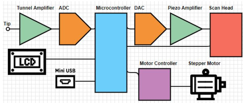
Figure 10: High level block diagram of tunnel current measurement device. Along with the power supply unit and keypad (not shown), these components complete the general architecture of the device. The 4x20 LCD displays basic information while built into the chassis. DAC-Digital to analog converter ADC-Analog to digital converter Modeled by Justin Jee using Digikey Scheme-It
