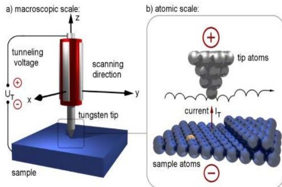
Figure 2: Illustration of a scanning tunneling microscope with a piezo tube scanner. [6]
