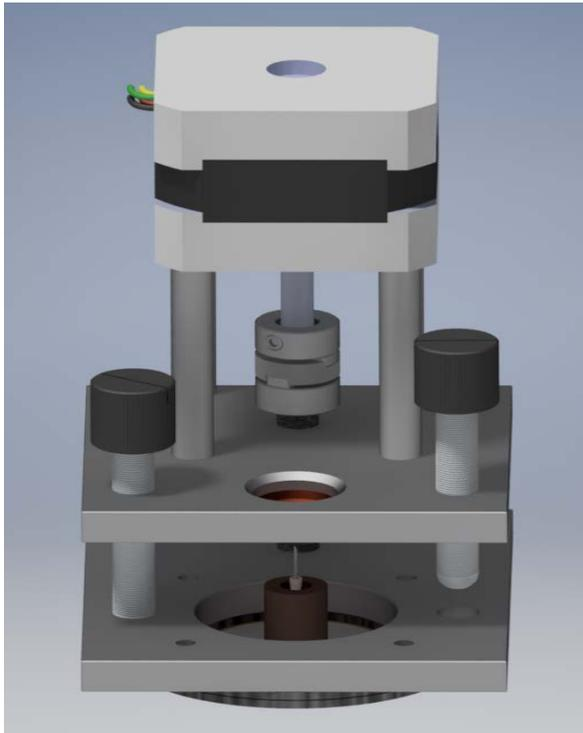
Figure 7: 3D model of the finished tunnel current device. This model describes the direction of the project, not necessarily the exact finished product. Designed by Justin Jee using SOLIDWORKS Student Edition.
