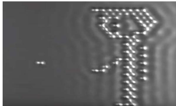
Figure 6: An image from the world's smallest movie, "A Boy and His Atom". IBM created this image using their STM. [10]
