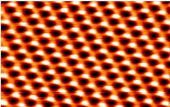
Figure 3: The structure of HOPG imaged with an STM. The proposed project uses this material as a substrate for measurements in atmospheric conditions. [7]
