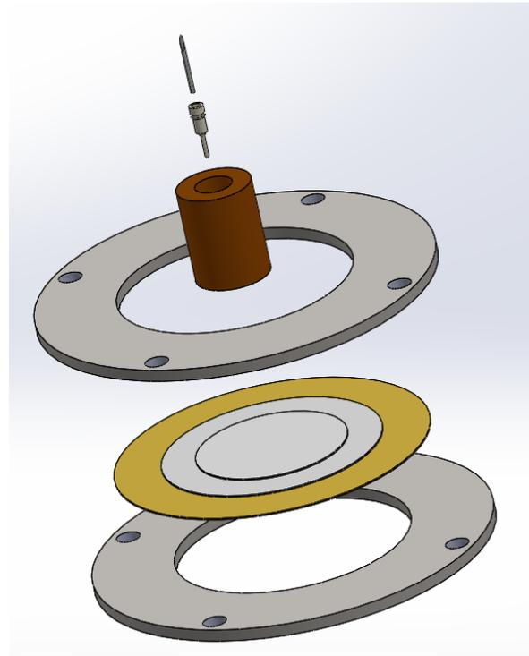
Figure 8: 3D model of the scan head subsystem. Parts shown from bottom to top: steel washer, piezo transducer, steel washer, phenolic standoff, DIP socket, tip. Designed by Justin Jee using SOLIDWORKS Student Edition.
