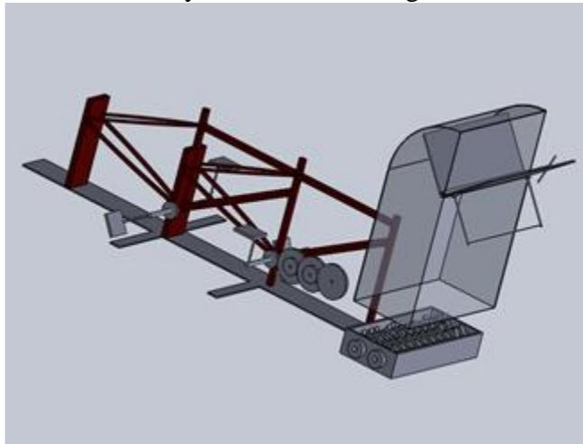
Figure 1. Rough design overview including mailbox-emulating safety mechanism, shredding devices, tandem bicycle framework, and drive train. Some aspects of the design have been left out of the model for simplicity.
