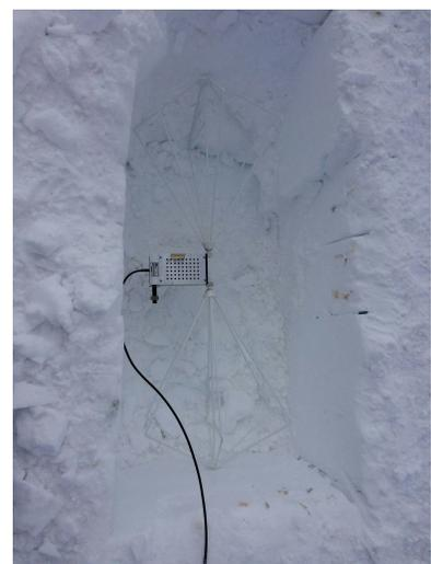
Fig. 1: Bicone antenna embedded in Antarctic ice for testing of ANITA III
