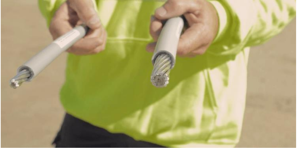
Figure 2.3.1: Example of Covered Conductor from SCE [15]
