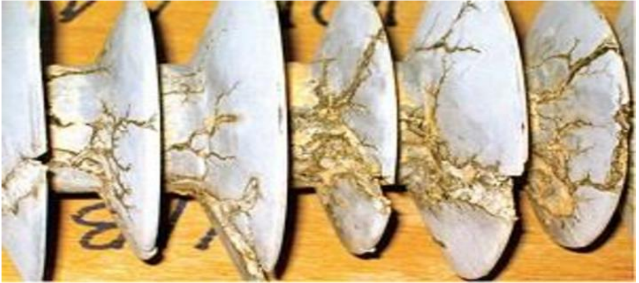
Figure 2.6.2: Electrical Tracking on Insulator
