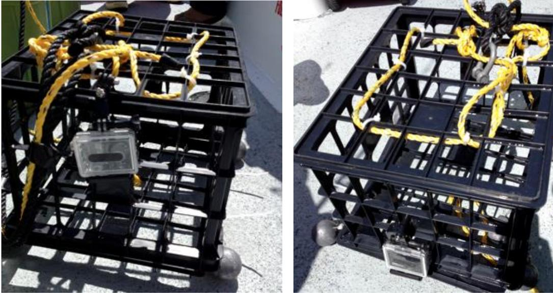
**Figure 2. Weighted Inverted Milk Crate Descending Device (Barotrauma Reliever).** Two GoPros are attached, one angled upward to view the fish during descend (left), and the other angled downward to view the fish upon release (right).
