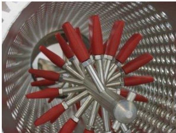
Figure 10. Internal picture of a destemmer. Copyrighted with permission by J. Lohr Vineyards & Wines 2017.
