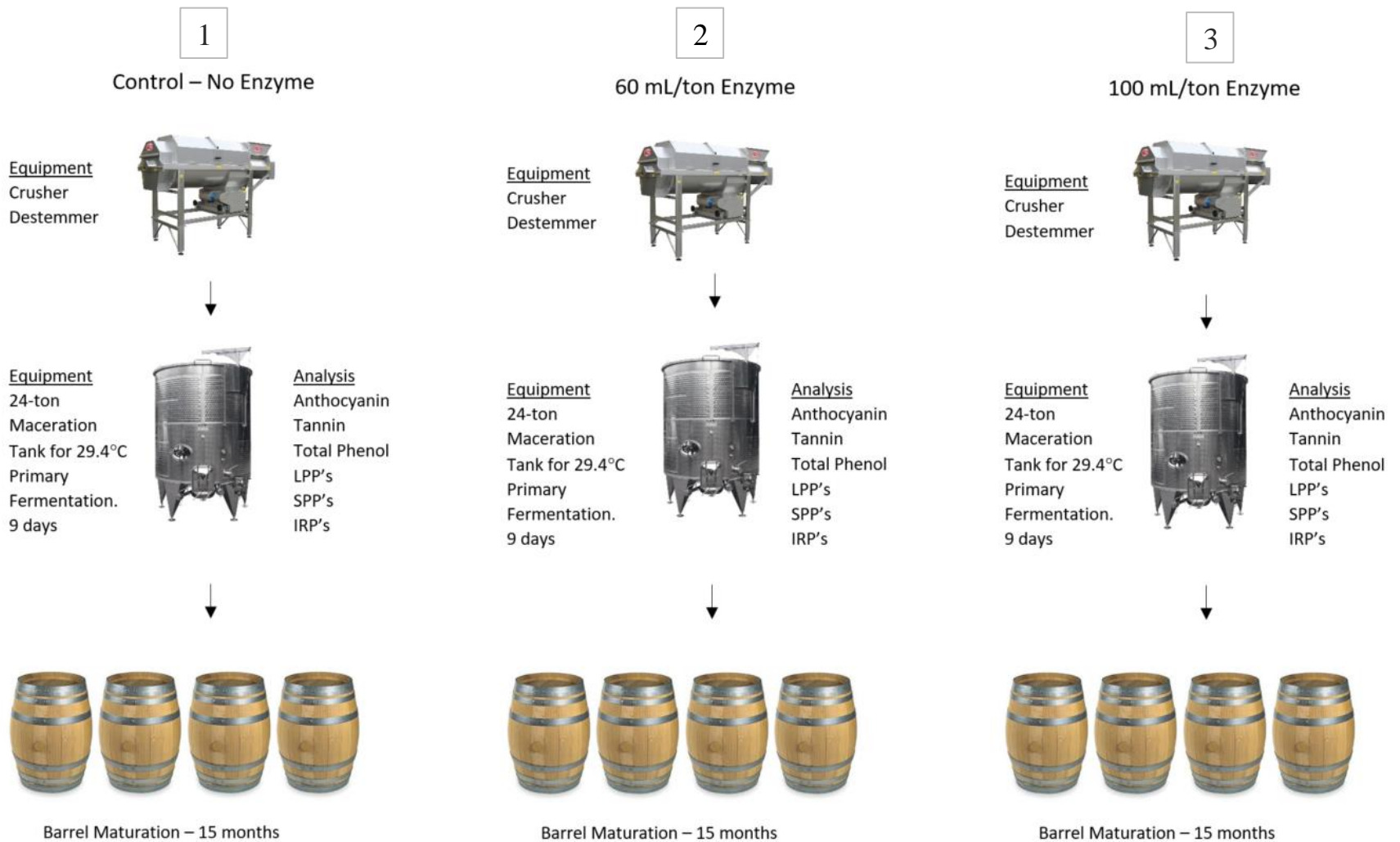
Figure 17. Schematic – Effect of enzyme application on phenolic compounds in the 2010 vintage. LPP's – long polymeric pigments, SPP's – short polymeric pigments, IRP's – iron reactive phenolics
