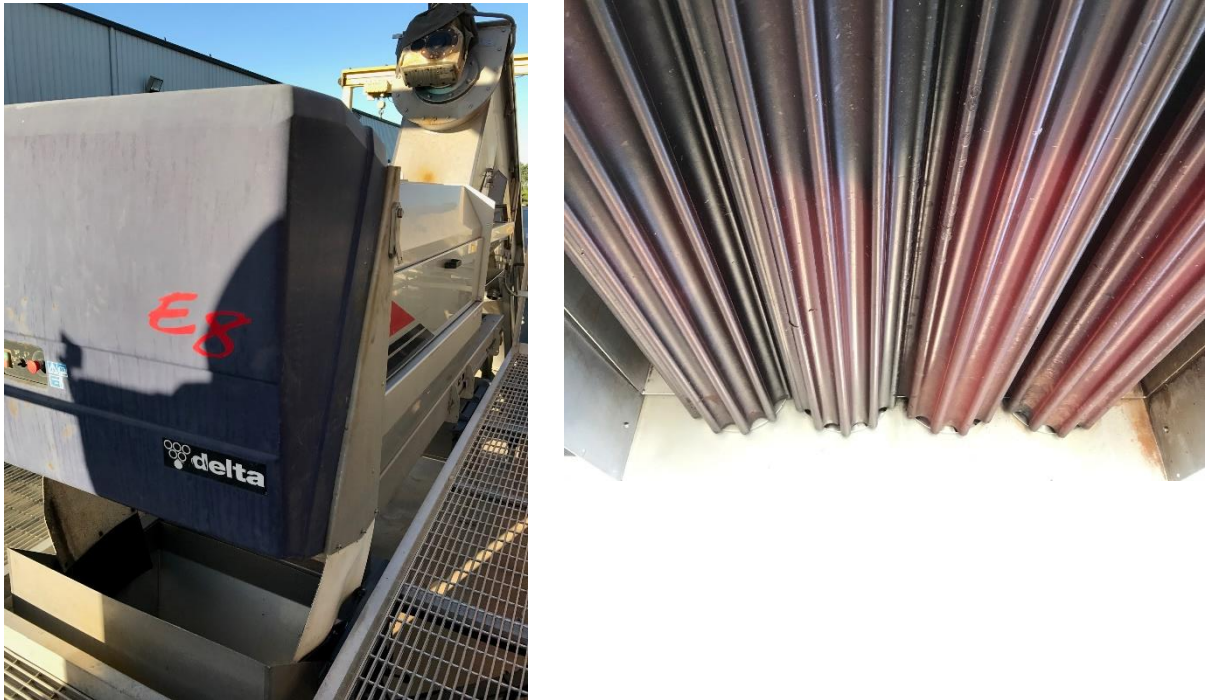
Figure 13. The Vaslin Bucher Delta E8 destemmer / crusher (left), and the rollers as viewed from below the destemmer / crusher (right). Copyrighted with permission by J. Lohr Vineyards & Wines, 2017.
