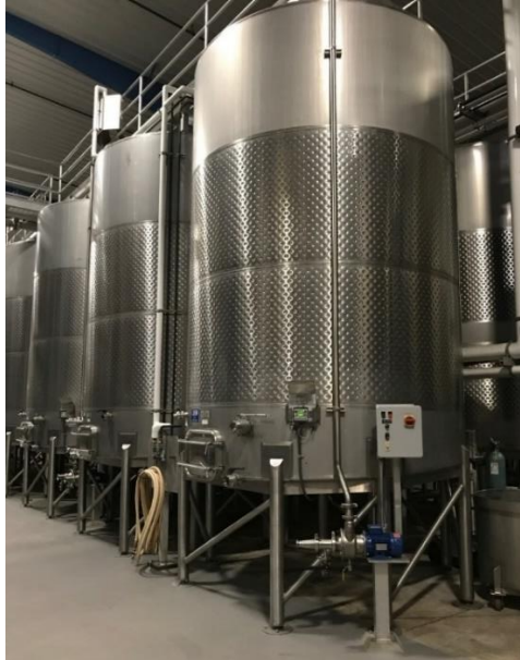
Figure 15. A fermenting tank with a designated pump for automated pump overs. Copyrighted with permission by J. Lohr Vineyards & Wines, 2017.
