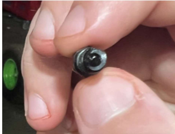
Figure 36. We determined that the bleed screw was unable to be installed deep enough to press into the sealing taper based on the non-uniform aluminum residue on the bleed screw taper. It appears that only about 2/3 of the taper was making adequate contact with the caliper-side taper.
