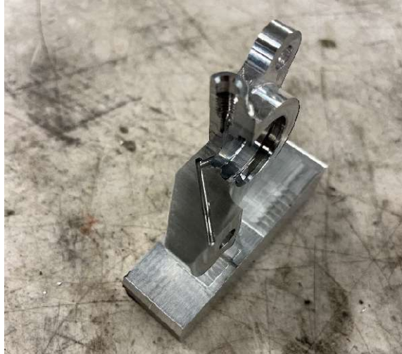
Figure 44. Caliper with cut made to reveal the internal fluid routing and sealing groove geometry. The surfaces were polished and optically inspected with a CMM.
