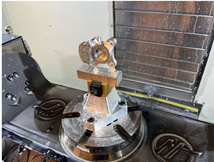
Figure 45. Finished caliper half held onto the machine with two tabs.
