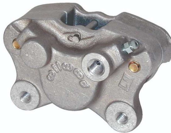
Figure 5. Wilwood PS1 caliper.
