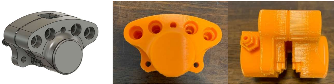
Figure 18. CAD and 3D Print of Concept Prototype.
