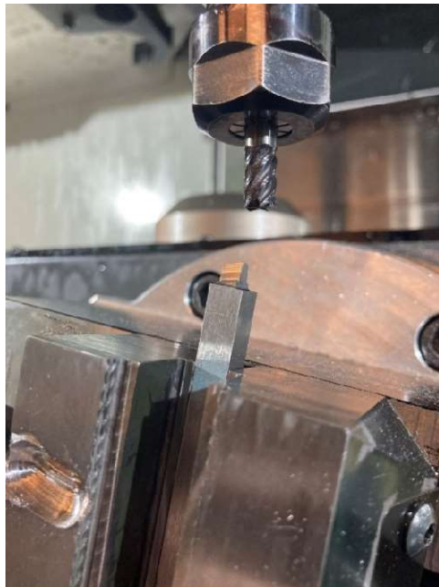
Figure 41. Machining of the inserts on a VF2-SS with TRT-160.
