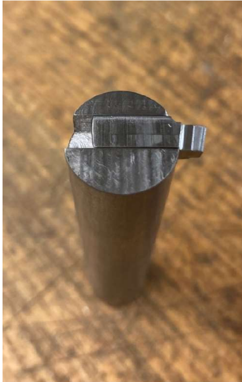
Figure 40. Grooving tool arbor manufacturing.
