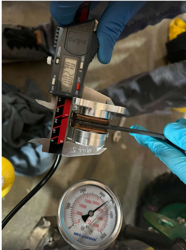
Figure 48. Caliper pressure and deflection testing. The calipers withstood 3400 psi and deflected a maximum of 0.027 inches.
