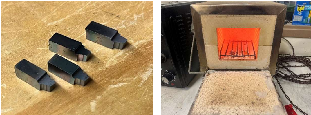
Figure 42. The finished inserts along with the oven used to preheat and soak (austenitize) the inserts.
