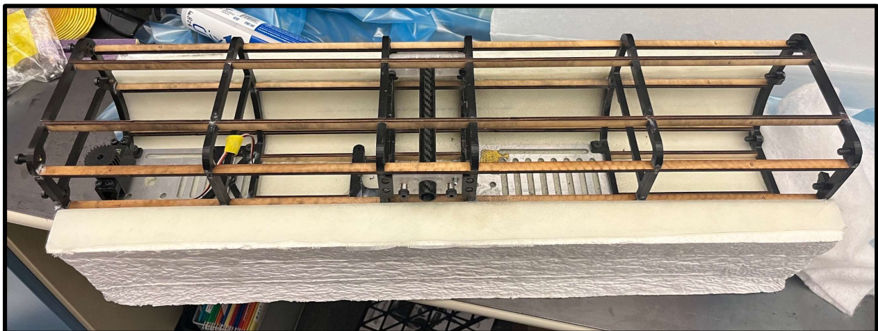
Figure 12. Internal Structure of the Fuselage After it was Adhered to the Bottom Skin Section
