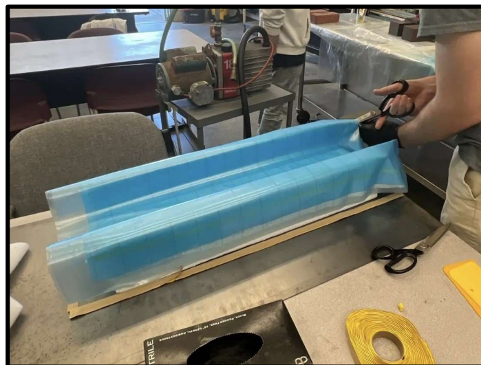
Figure 10. Preparing Fiberglass in the Fuselage Mold
