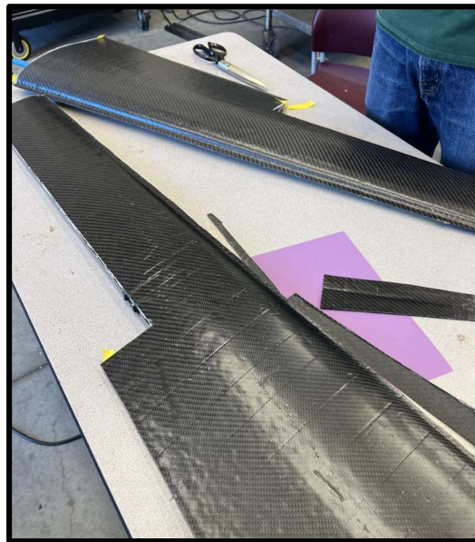
Figure 11. Partially Completed Wings After the Top and Bottom Carbon Fiber Skin Sections were Adhered to the Internal Structure of the Wings
