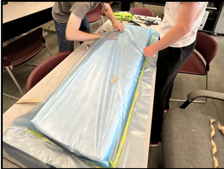
Figure 9. Placing the Carbon Fiber in a Vacuum Bag After the Wet-Layup
