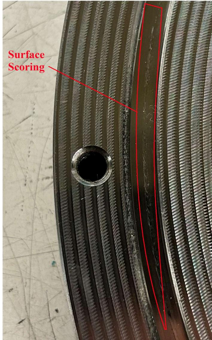
Figure 5.2. Wear on the sealing surface of the plate after cyclic load testing.
