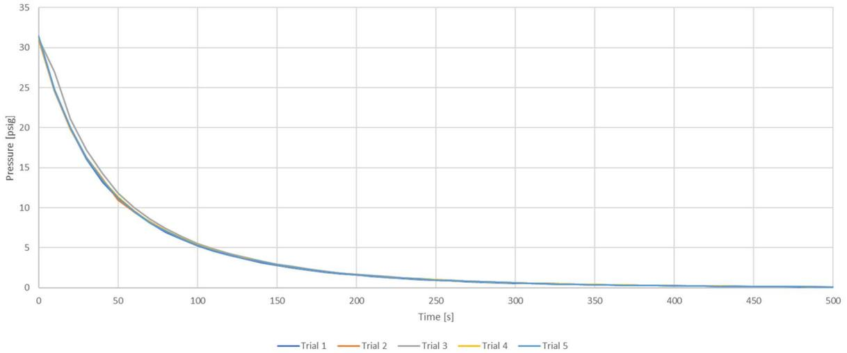
Figure 4.3. Characteristic pressure decay test results.
