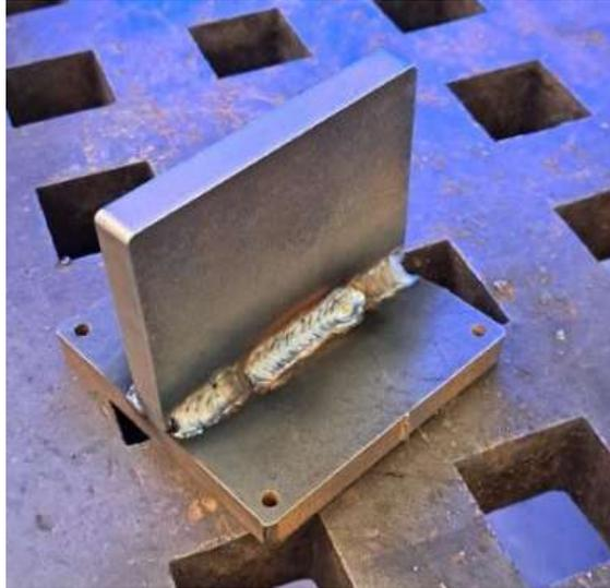
Figure 3.8. Welded fixture for load frame machine.
