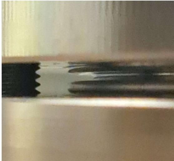
Figure 3.11. Compressed seal between the two plates.
