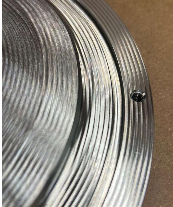
Figure 3.5. CNC milled E-seal groove surface finish.
