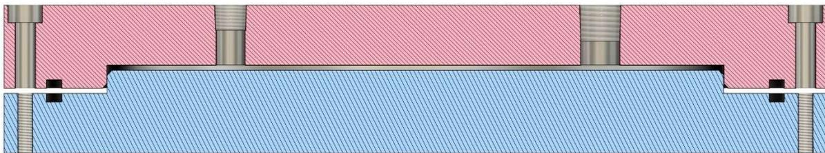
Figure 5. A Section View of the Test Prototype Showcasing the Small Internal Volume (Gray Area Between Plates) to Pressurize for Testing
