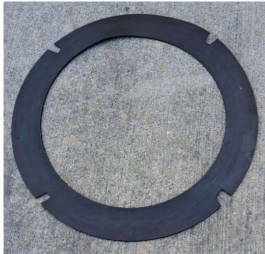
Figure 3.9. Additional baseline rubber gasket.
