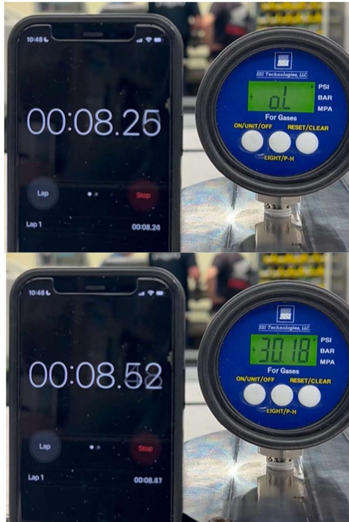
Figure 4: The Pressure Gauge Overloaded at about 30psi While Testing.
