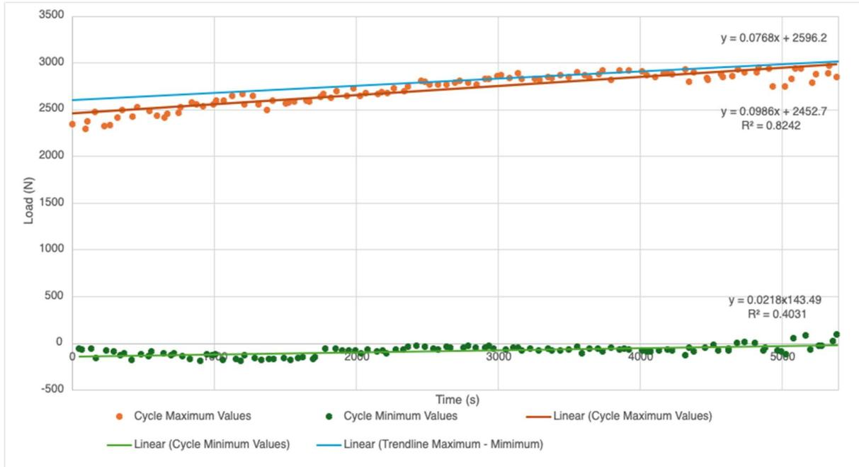
Figure 4.5. Force in Newtons required to deflect the seal by 0.030 inches. Peak compression and tension values shown.
