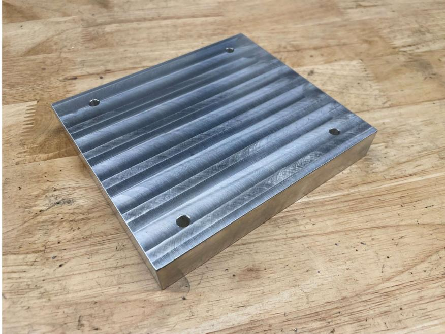
Figure 3.6. The fixture plate used to hold stock during CNC machining.
