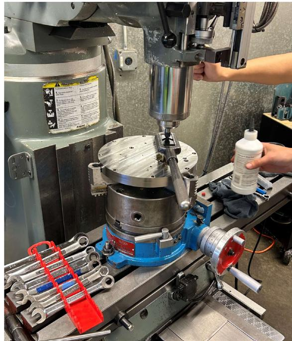
Figure 3.4. Tapping the top plate on the Bridgeport mill.
