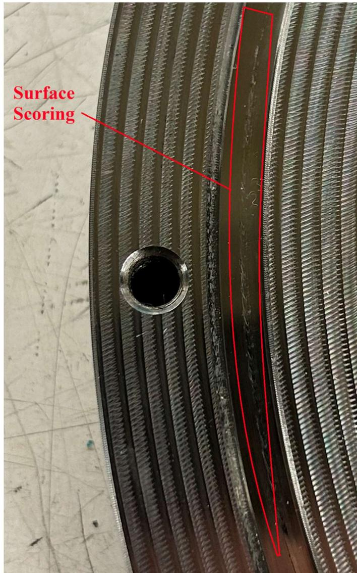
Figure 7: Surface Scoring on the Sealing Surface of the 17-4 Stainless Steel Plate
