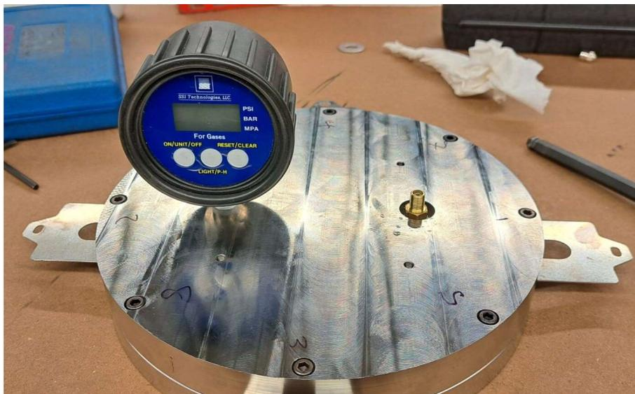
Figure 3.1. Prototype test rig completed assembly.
