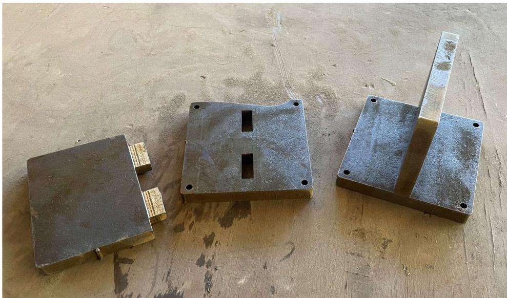
Figure 3.7. Post machining pre-welding of load frame attachment points.
