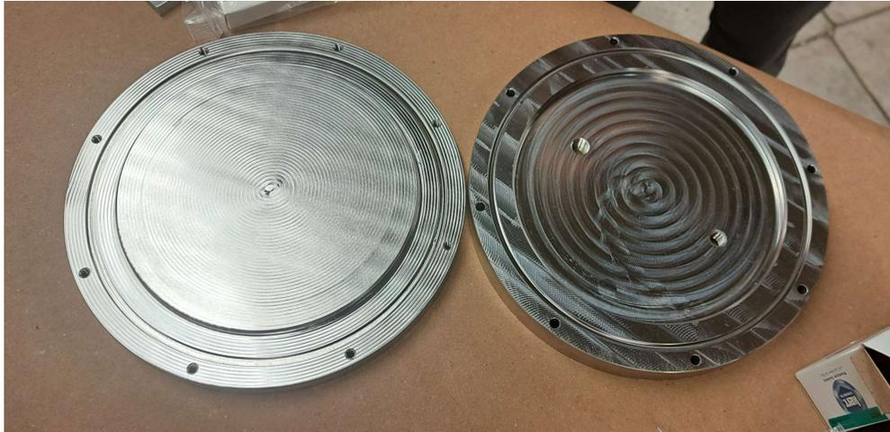
Figure 3.3. Post CNC milled test rig plates.
