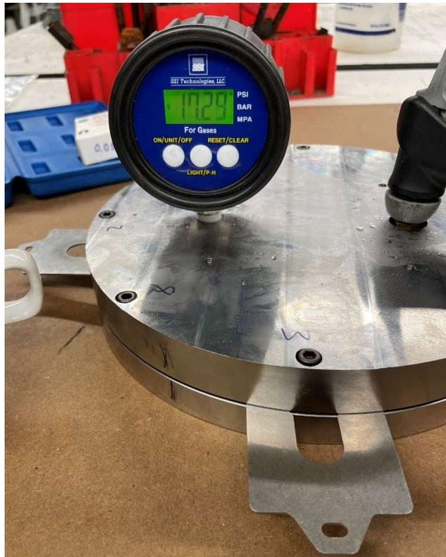
Figure 4.1. Leak testing setup. The bike pump pressurizes, and the digital gauge reads cavity pressure.
