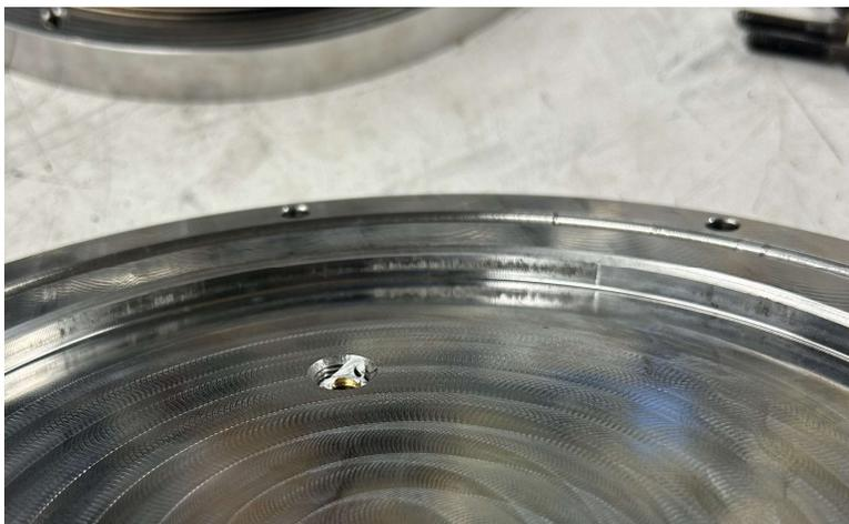
Figure 5.1. Wear on the inside of the test rig top plate where it contacted the bottom plate during cyclic loading.
