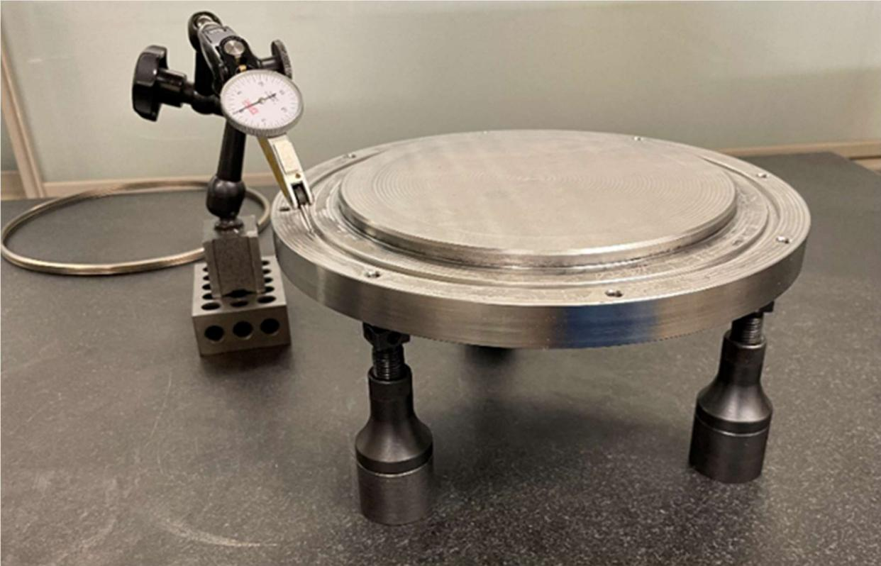
Figure 2. E-Seal Groove Flatness Inspection
