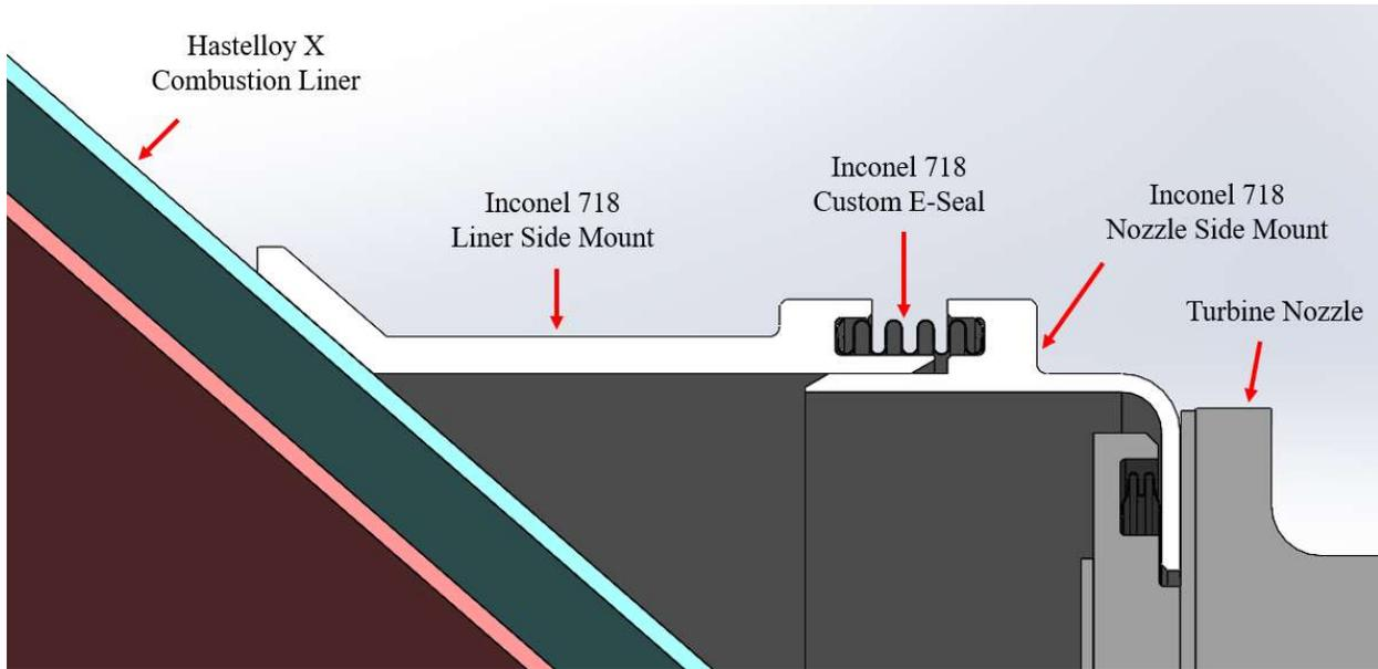
Figure 22.11. Section view of the E-seal assembly in-place of the current fishmouth.
