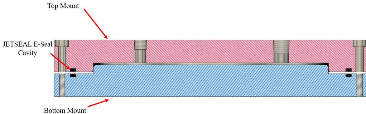
Figure 2.3. Section view of the functional prototype test rig.
