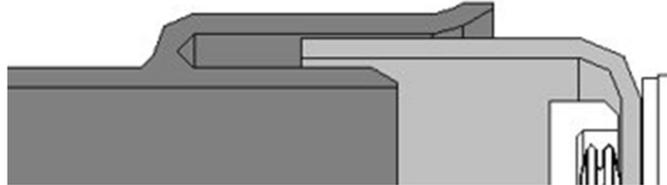
Figure 1.1. Fishmouth seal on Solar Turbines' T250 combustion liner to stage 1 nozzle [1].
