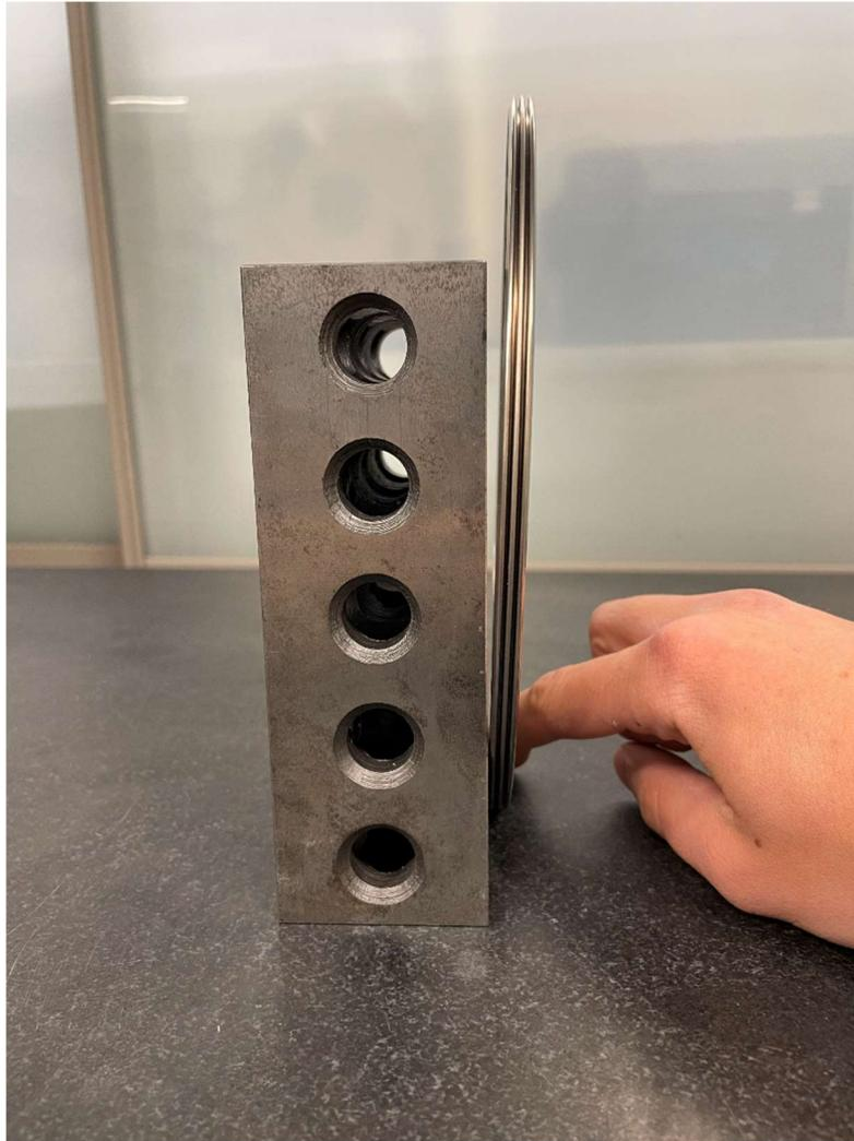
Figure 6. The Seal Held Flat on a Surface Plate Next to a One-Two-Three Block Showcasing the Seal's Asymmetry.
