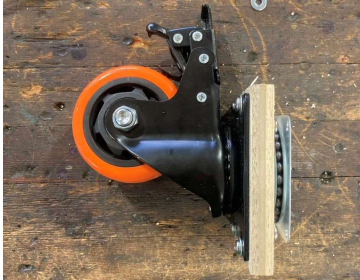
Figure 8. Addition of Turntable Bearings Between the Base and Caster Wheels
