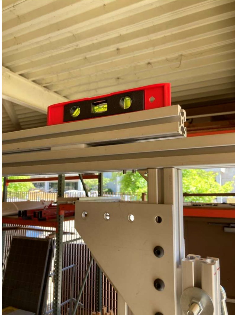
Figure 7. Addition of Beams Across the Top of the Vertical Beams. This photo has the corner plate bracket detached from the horizontal members to show the joining in more detail.
