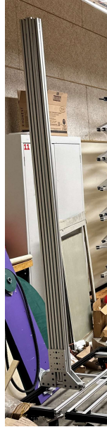
Figure 19. The Vertical Beams mounted to the rest of the Moving Base Subsystem.
