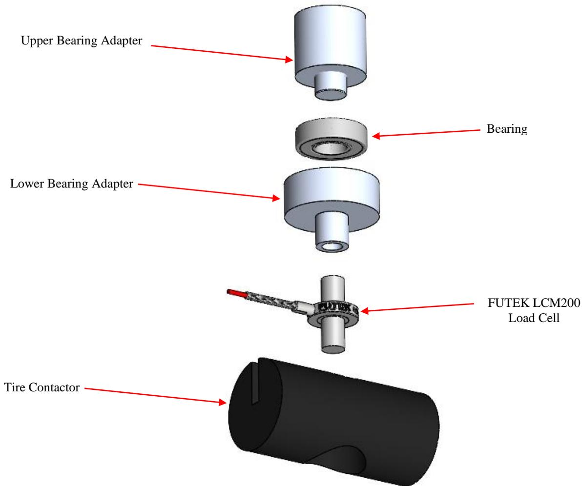
**Figure 2:** Exploded view of new load cell assembly.
