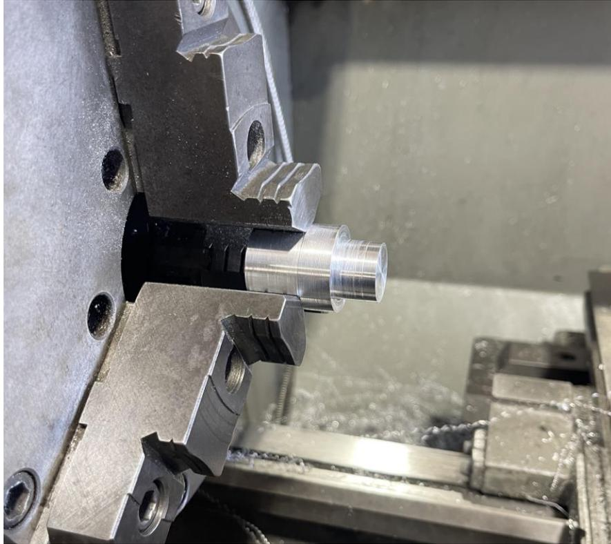
*Figure 4:* Upper bearing adapter in the lathe chuck during the first operation.
