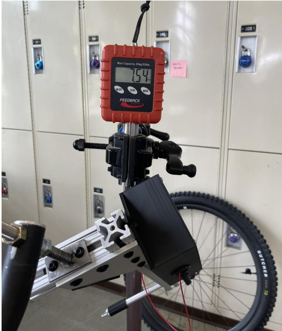
*Figure 1111:* Picture of device weighed using a digital bike scale.
