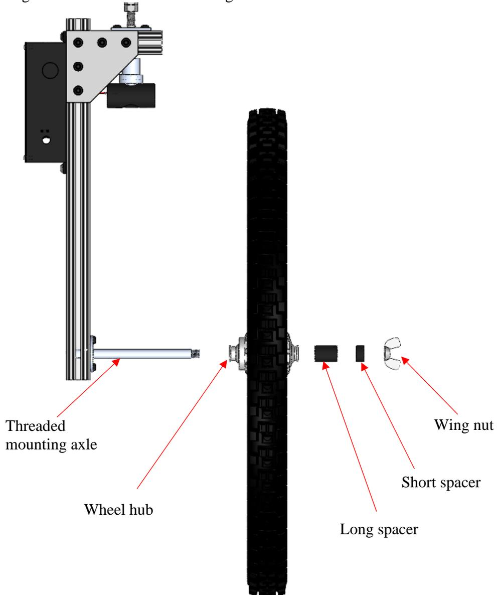
**Figure 13:** Exploded view of the wheel mounting assembly.
