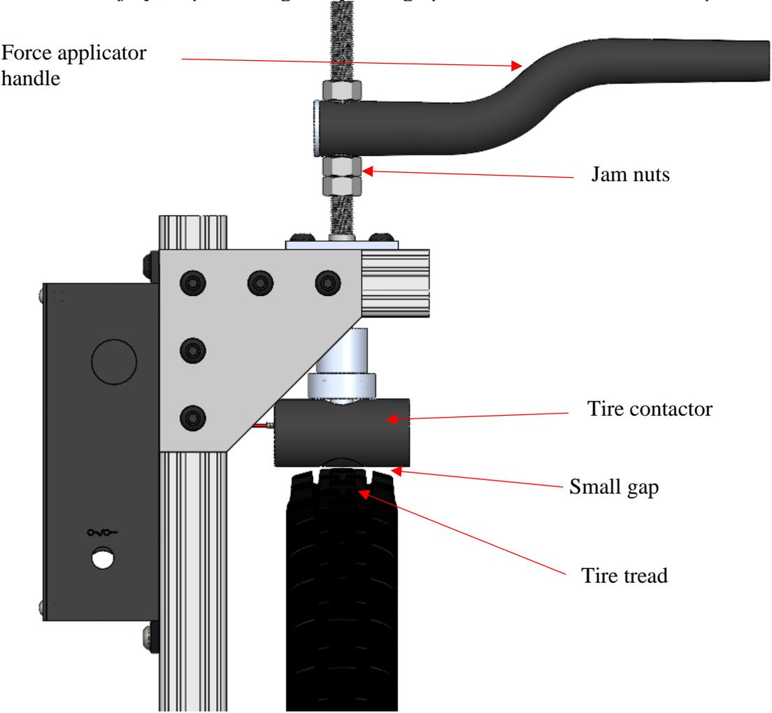
**Figure 7:** Tire contactor in position directly above the tire tread, ready for data collection.
