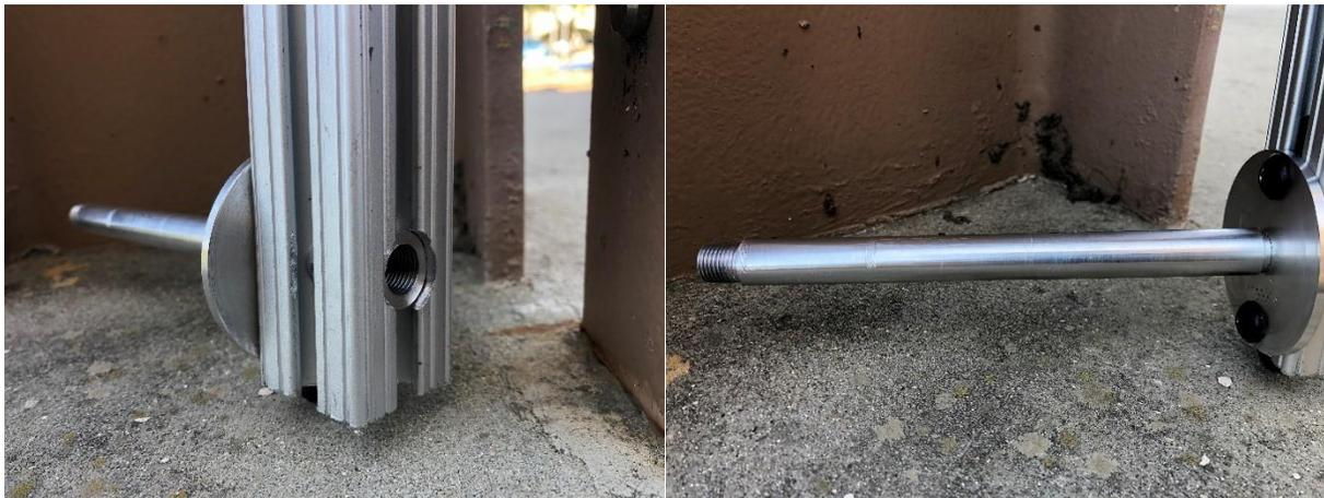
**Figure 77:** Wheel axle and threaded insert components.
