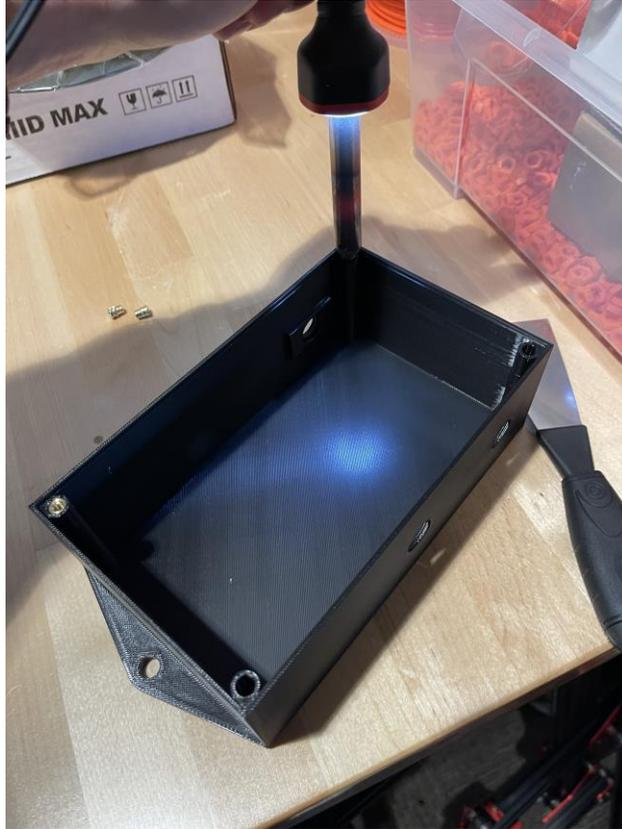
**Figure 6:** Using a soldering iron to set the heat-set threaded inserts into the DAQ housing.
