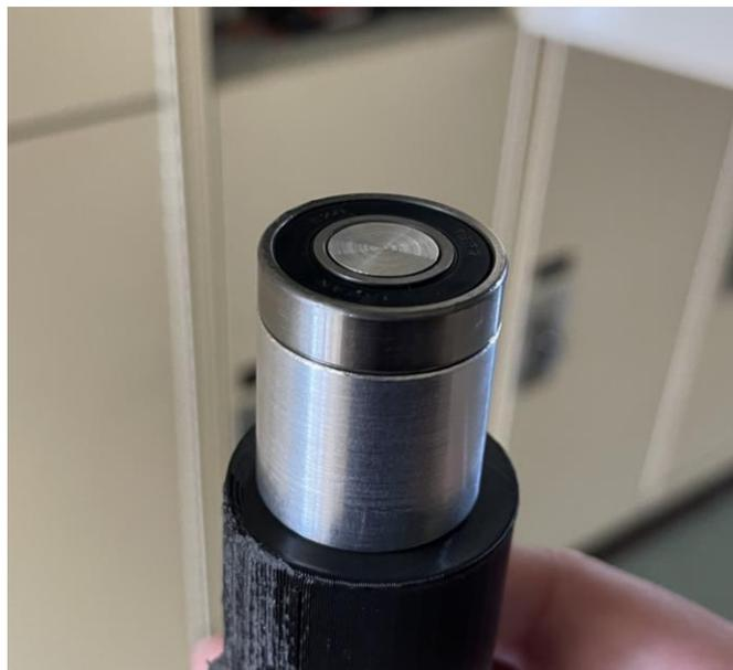
**Figure 8:** Ball bearing pressed onto the upper bearing adapter.
