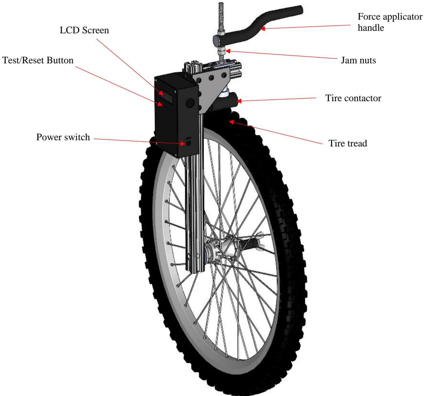
**Figure 6:** Isometric view of the tire spring rate measurement device with labeled components of operation.
