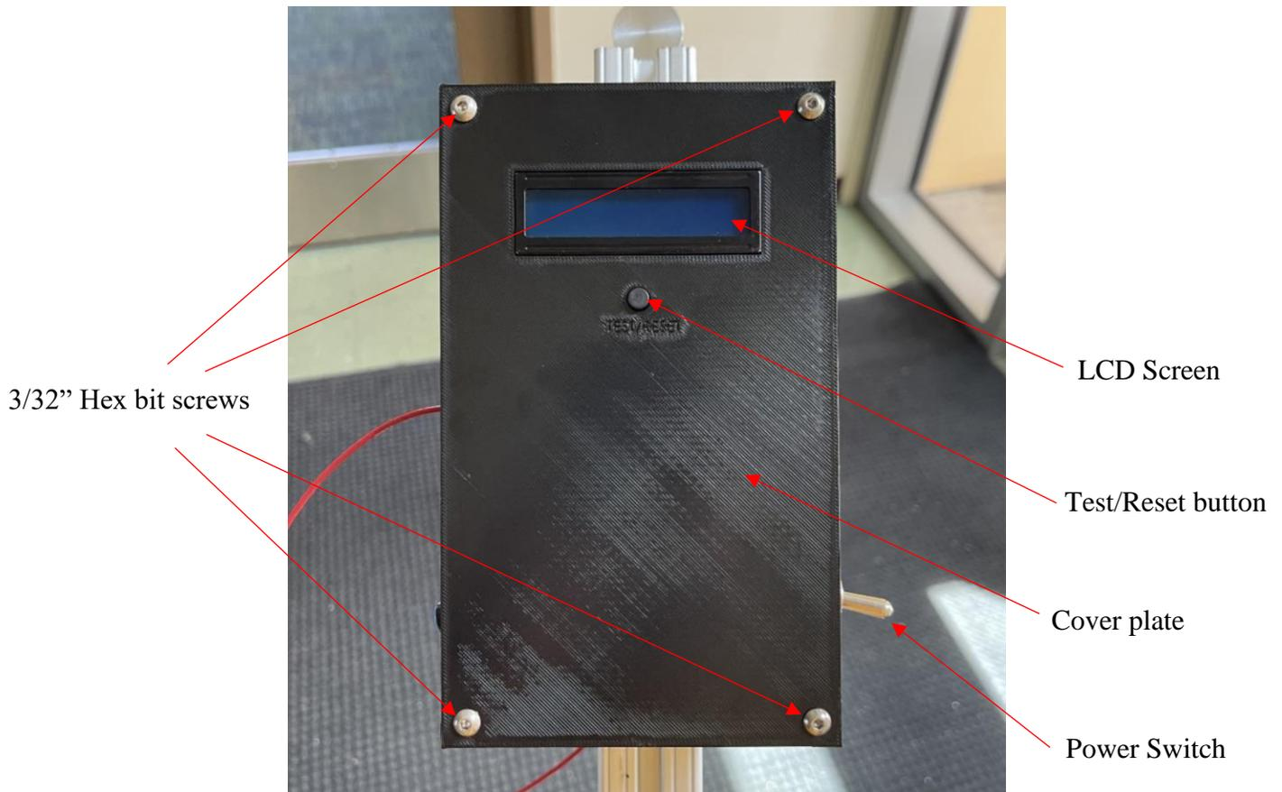
**Figure 4:** Electronics housing cover plate.
