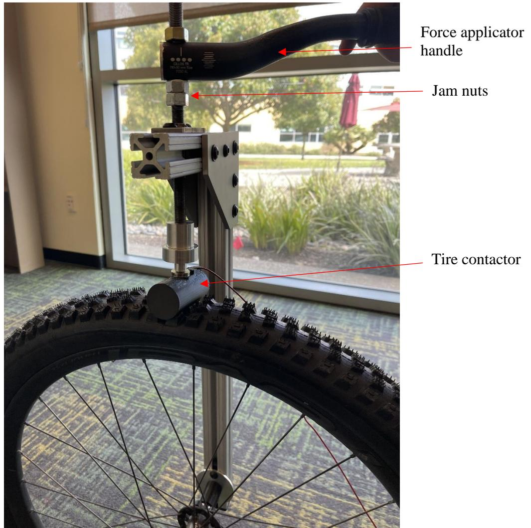
**Figure 8:** Compression of the tire after the fixed displacement set by the lock nuts has been reached.
