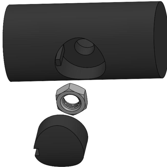
**Figure 3:** Close up view of the tire contactor assembly.
