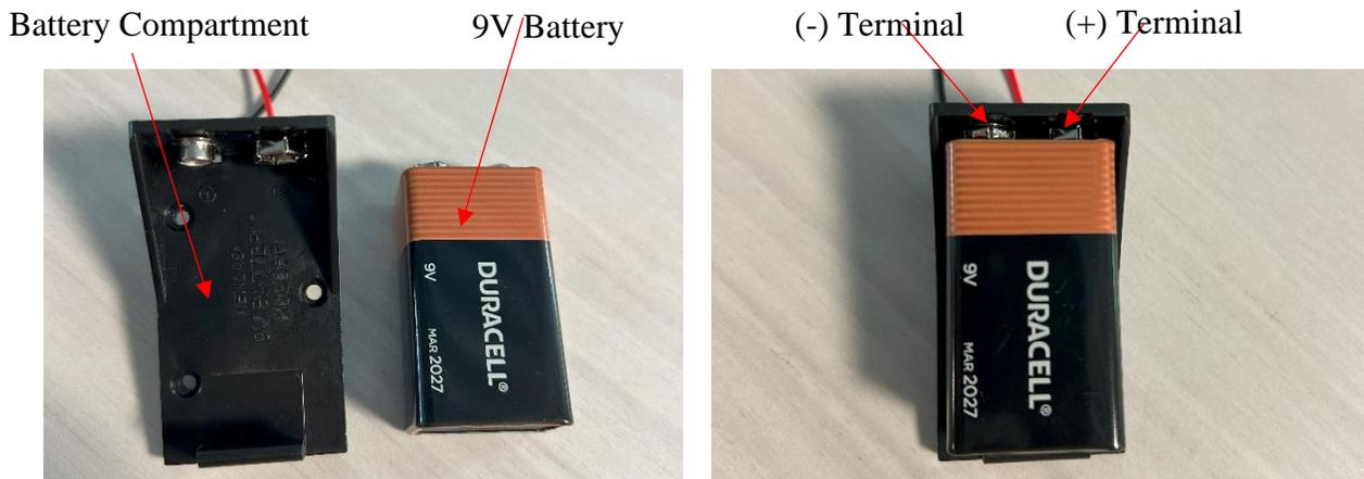
**Figure 5:** Installation of the 9V battery.
