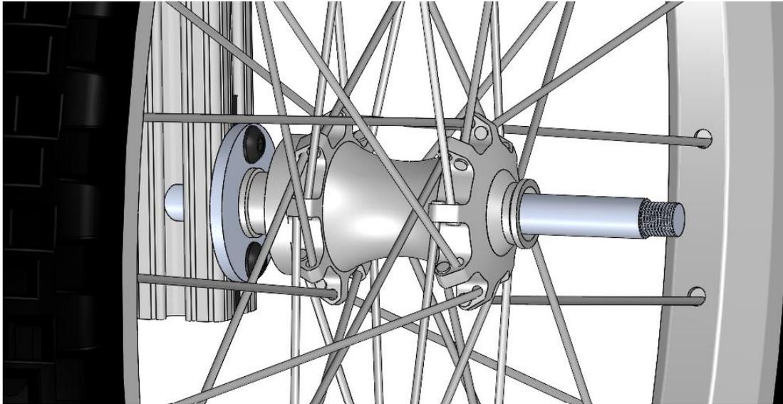
**Figure 2:** Zoomed in view of the wheel hub pressed against the spacer on the axle.
