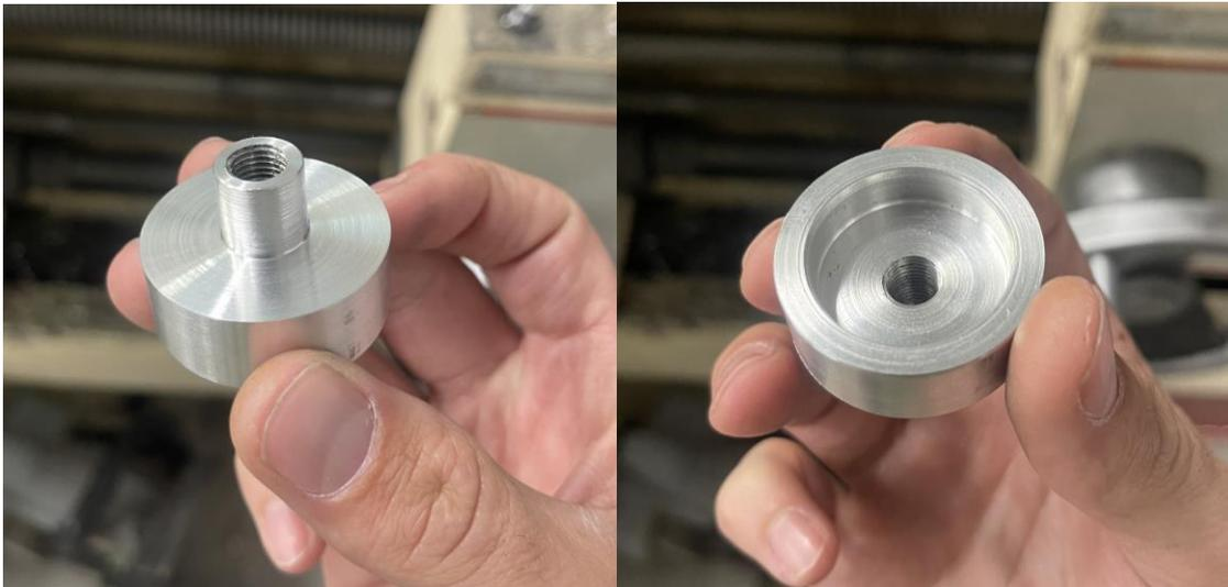
**Figure 5:** Lower bearing adapter top and bottom sides after manufacturing was complete.
