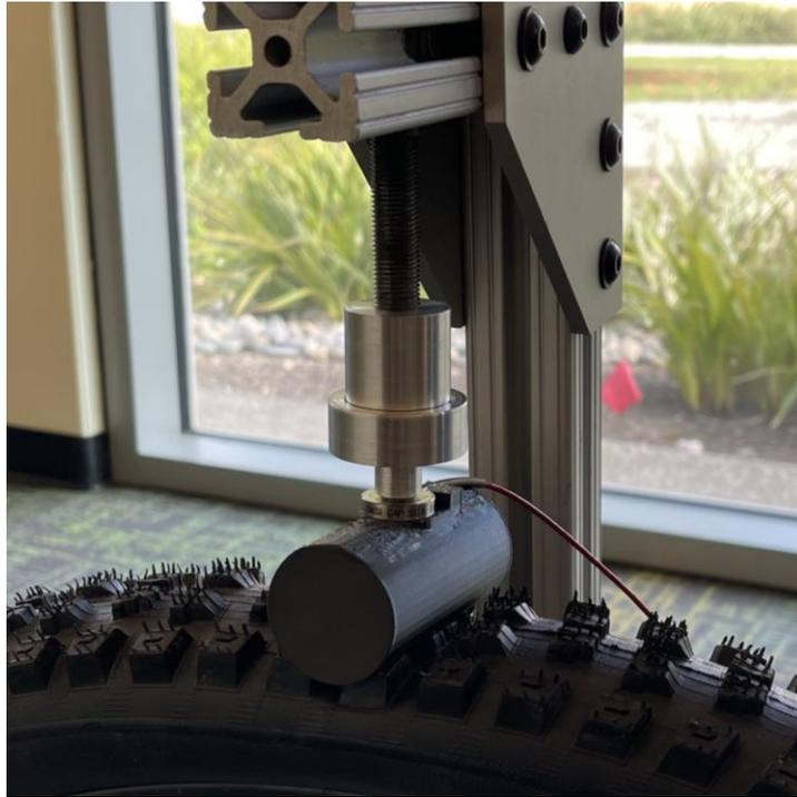
*Figure 9:* Completed lower section of the force application assembly.
