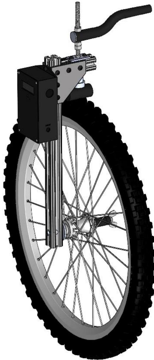
*Figure 1:* Isometric view of final tire spring rate measurement device.
