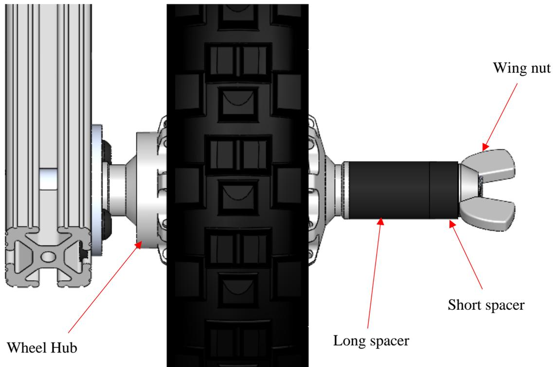
**Figure 3:** Side view of the complete wheel mounting assembly.
