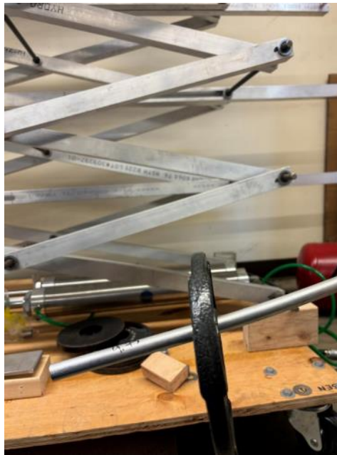
Figure 18. Applied 2.5 lb weight to edge of D-ring.
