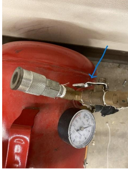
Figure 3A: Silver valve handle used to control the airflow into pistons.
