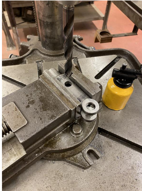
Figure 10. Modified piston clevis next to the drill press set up used.
