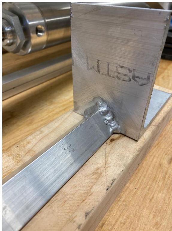
Figure 9. Close-up of V-groove track weld
