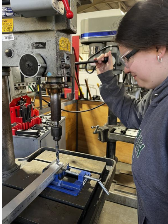
Figure 1. Drilling holes into the scissor lift links.
