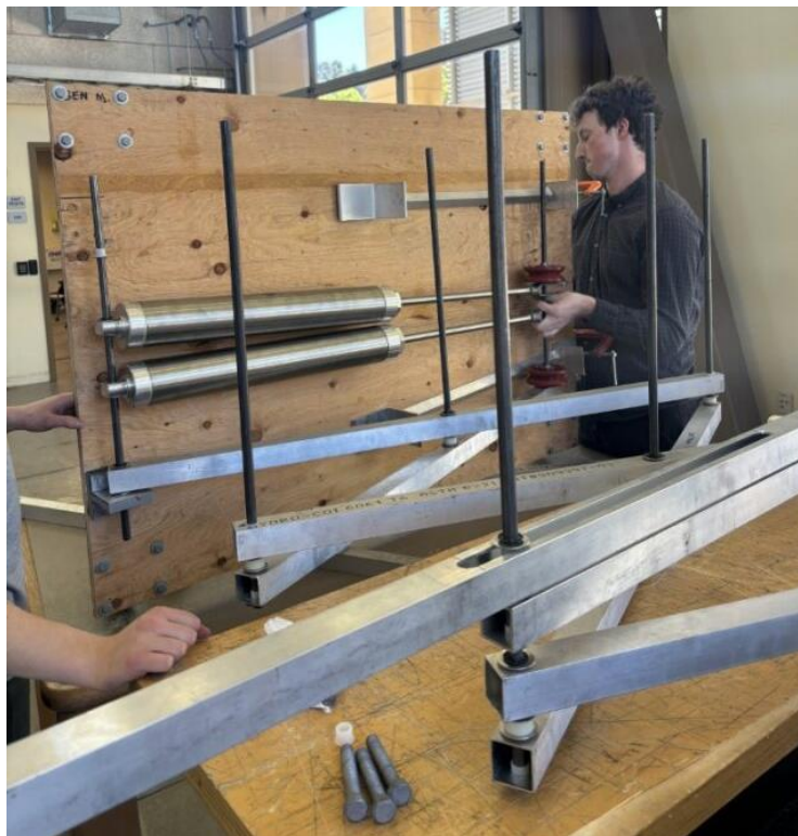
Figure 15. Attaching the scissor lift to the base platform assembly.
