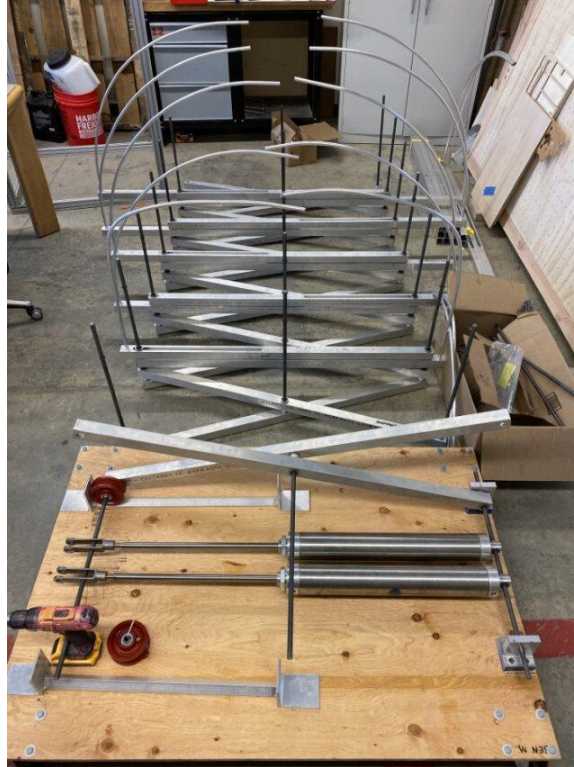
Figure 13: The scissor lift assembly and base assembly side by side.
