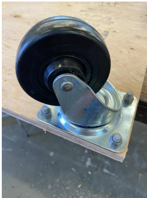
Figure 6. Swivel caster wheel bolted in the corner of the plywood base.
