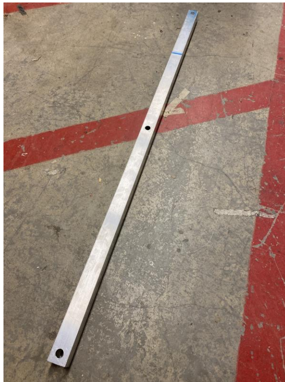
Figure 2. Cut and drilled scissor lift link.
