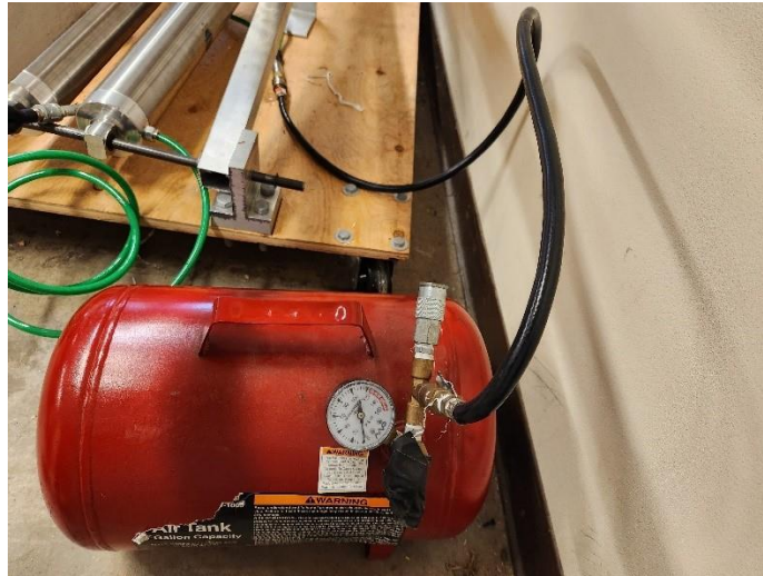
Figure 1A: 5-gallon air tank with dial pressure indicator.
