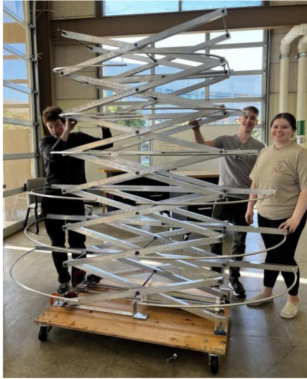
Figure 16. Completed Christmas tree frame assembly.
