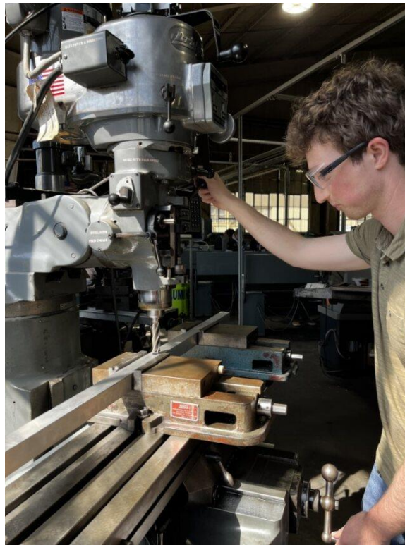
Figure 3: Manual Milling Slots into D-ring Links
