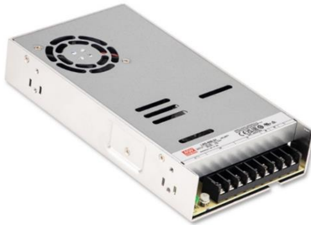
Figure 10 – The LRS-600-36 power supply from MEAN WELL, sourced off of DigiKey. Capable of providing 600W at 36V. Takes an input of 110VAC or 220VAC if configured properly.
