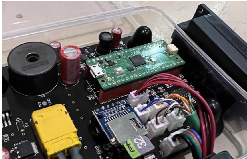
Figure 111 – Fully seated Pico. The enclosure is now ready for insertion into a tile.
