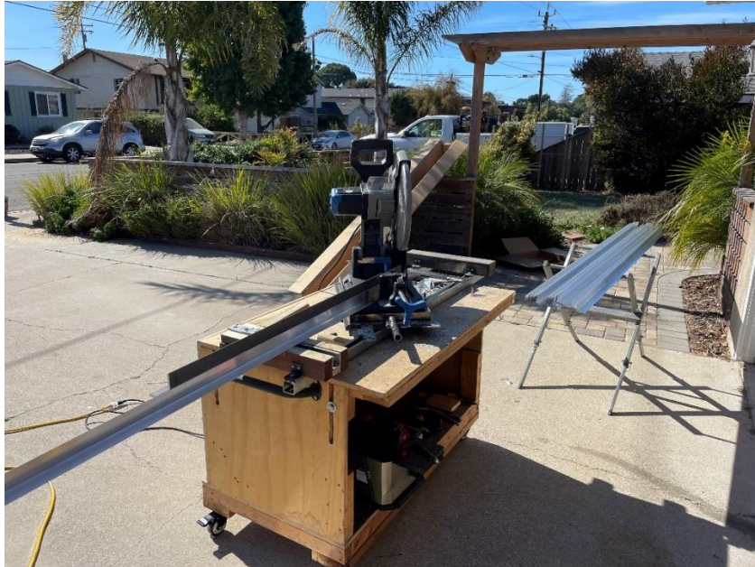
Figure 47 – Layout of each aluminum section for initial bevel cut.
