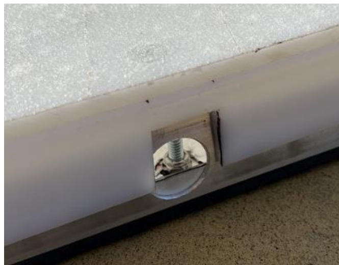
Figure 21 – Wire hole and cutout on the angled side of the Verification Prototype. In the final design, the rectangular cutout was updated to a semi-circular hole for ease of manufacturing.
