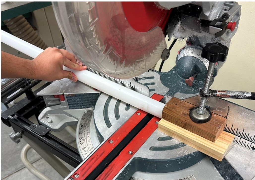
Figure 62 – Stock UHMW rod butted against stop and held in place to cut to length.
