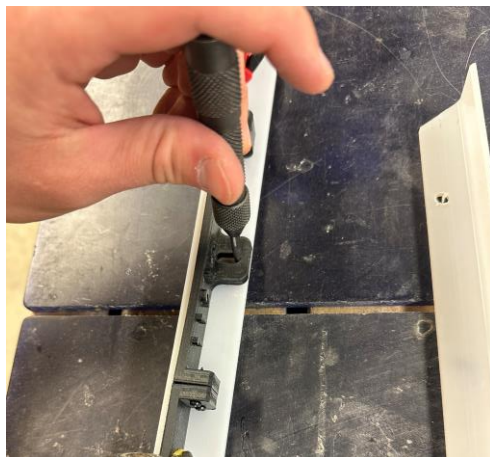
Figure 28 – Using a marking jig to center punch the edges of a slot.
