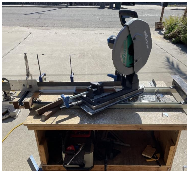
Figure 48 – Each section was flipped and cut at 37.5 degrees using a limit stop.
