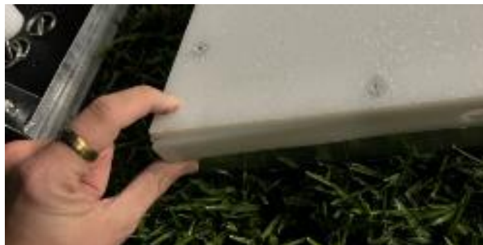
Figure 152 – Lid placement technique. Usually performed with two hands, the thumb is pushing inwards on the aluminum while the forefinger is pushing downwards. When performed with two hands, this move is especially effective on corners and at the center of the sides.
