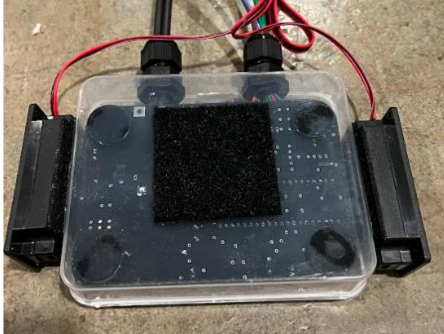
Figure 82 – Enclosure with Velcro placed on underside.
