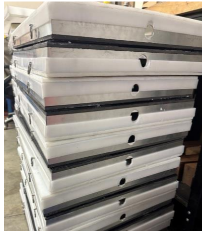
Figure 160 – Tiles stacked in alternating method so grip tape stacks against grip tape and rubber against rubber.
