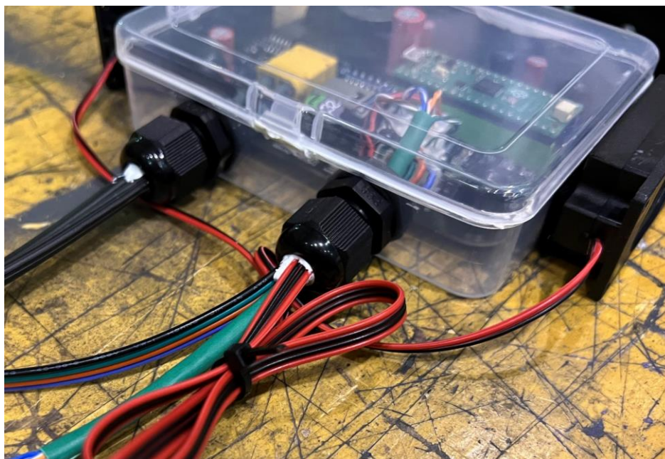
Figure 9 – Electronics enclosure with waterproof glands installed and sealed. The final board is also installed and the speakers are mounted to the side using Velcro.
