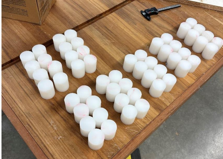
Figure 63 – Cut UHMW rods grouped into 8 pieces.
