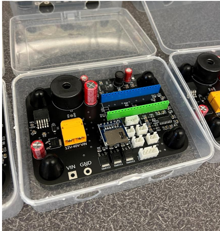
Figure 89 – Fully assembled PCB in an unfinished enclosure.
