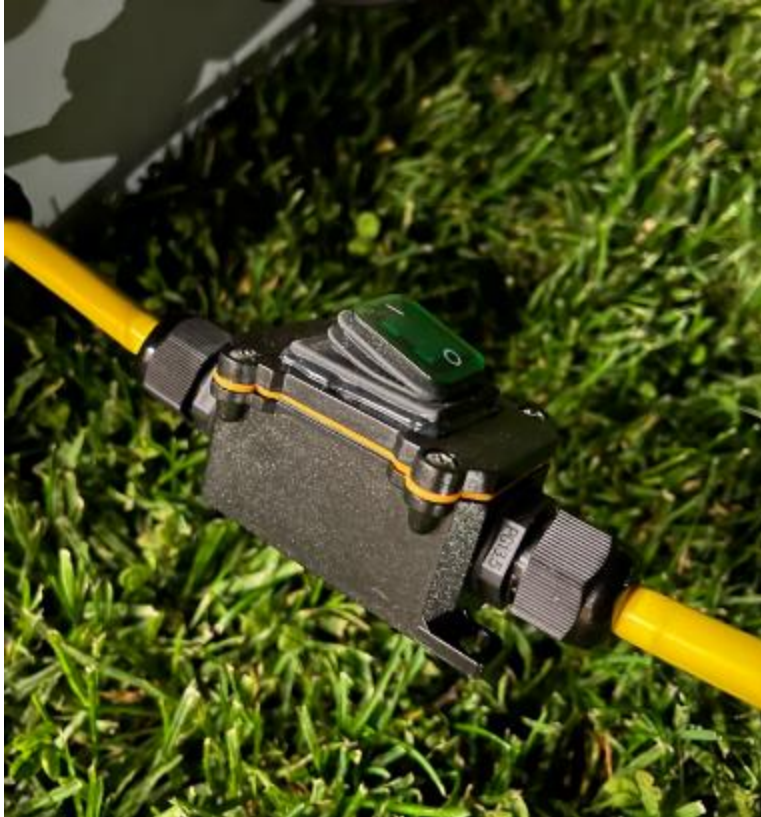
Figure 119 – Power supply’s green switch turned to the “O” position. The power supply should always be off when setting up or tearing down tiles.
