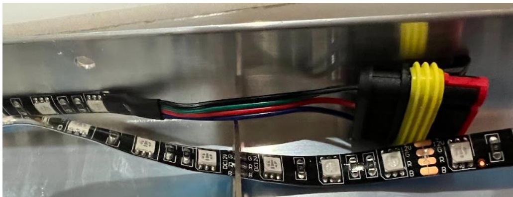
Figure 79 – Trimming the LEDs with scissors at a silver line. If needed, the LEDs can be trimmed at the bronze line seen near the right of the image.
