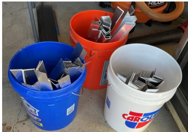
Figure 23 - Cut and categorized aluminum 90 degree angles waiting to have holes marked and drilled.
