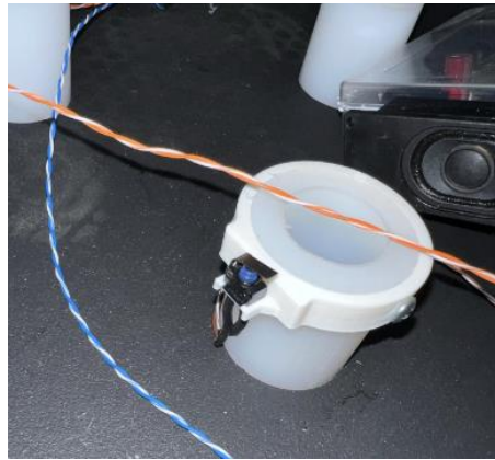
Figure 145 – Limit switch in place on limit switch mount, resting on internal support.
