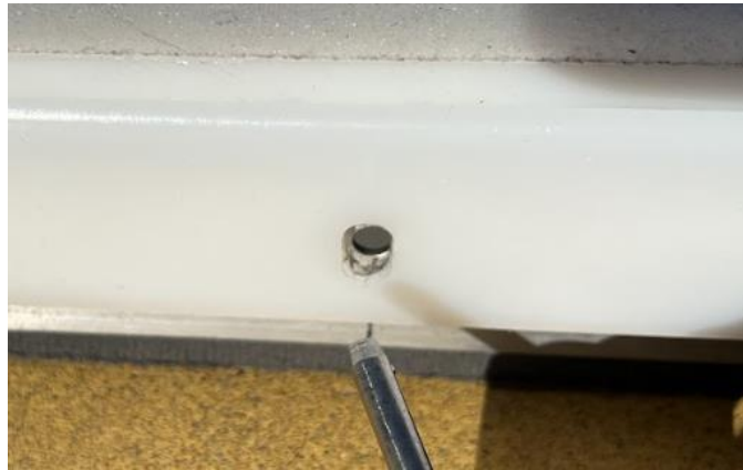
Figure 20 – Pinhole in bottom siding viewed through slot in top siding. In the final design, this slot was changed to a 0.5 inch hole for ease of manufacturing.
