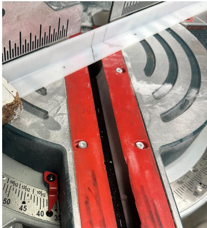
Figure 57 – UHMW 90-degree angle stock being cut at a 37.5-degree angle on the miter saw.
