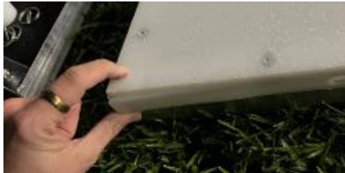
Figure 136 – Lid placement technique. Usually performed with two hands, the thumb is pushing inwards on the aluminum while the forefinger is pushing downwards. When performed with two hands, this move is especially effective on corners.
