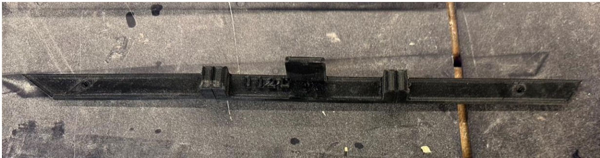
Figure 25 – Example marking jig, used for marking, punching, and scribing lengths, angles, holes and slots in the 90 degree angles.
