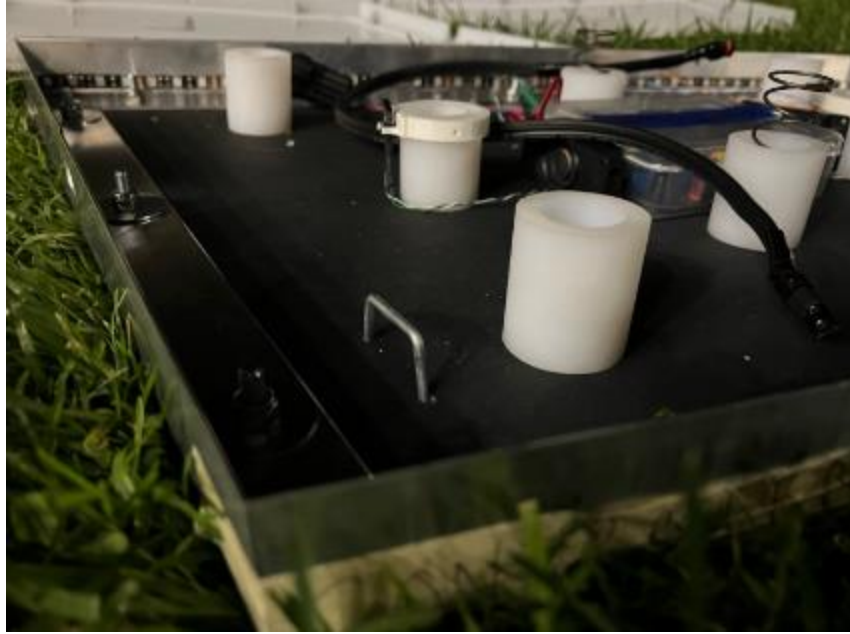
Figure 129 – Ensure stakes are more than halfway below the tile's height.
