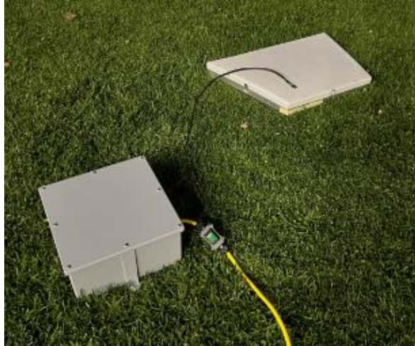
Figure 121 – “Controller” tile set up in range of the power supply’s black cable. After placing the “controller” tile here, the external label may be removed, though if done, needs to be replaced upon teardown.
