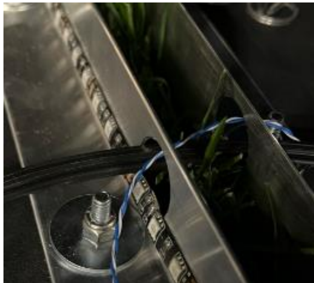
Figure 132 – First, feed through Tile B’s (on the right) blue and long, black cable through both wire holes, meeting on their adjacent side. The blue connector should pass through first due to its size.
