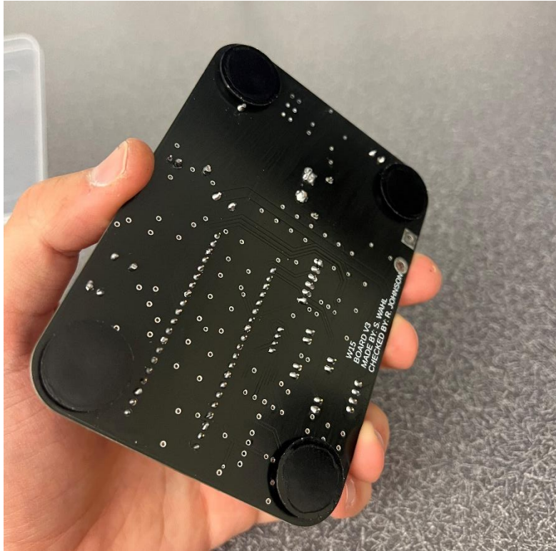
Figure 97 – PCB with internal rubber standoffs pushed through the mounting holes.
