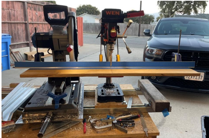
Figure 51 – Drill press station assembled with fence to maintain consistent hole locations.
