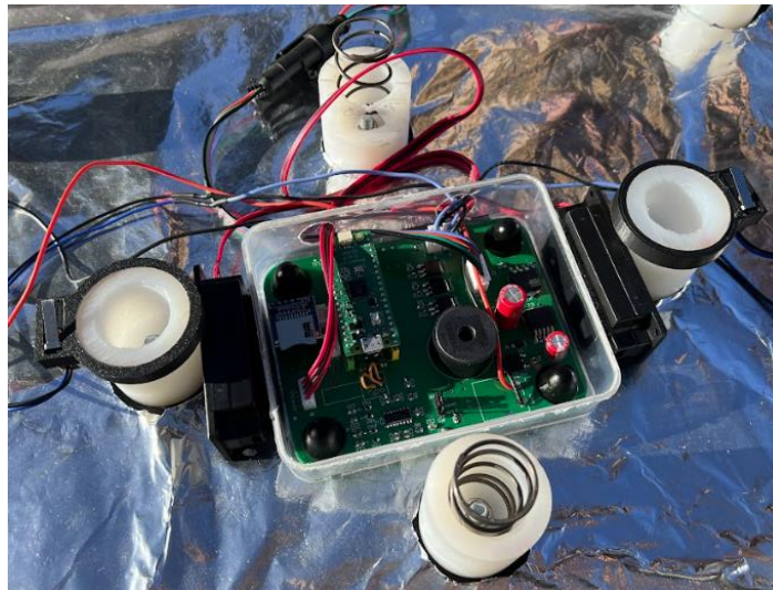
Figure 16 – Closeup of Test Board v2 as seated in the Verification Prototype. Note how the limit switches and their mounts differ from the version presented in Section 2.1.
