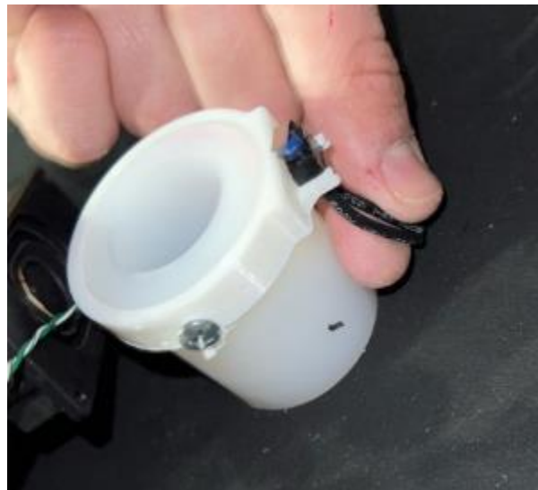
Figure 156 – Pressing on the switch's body to insert it onto the rails. Ensure that the switch's metal arm points up towards the long side of the tile when inserted.
