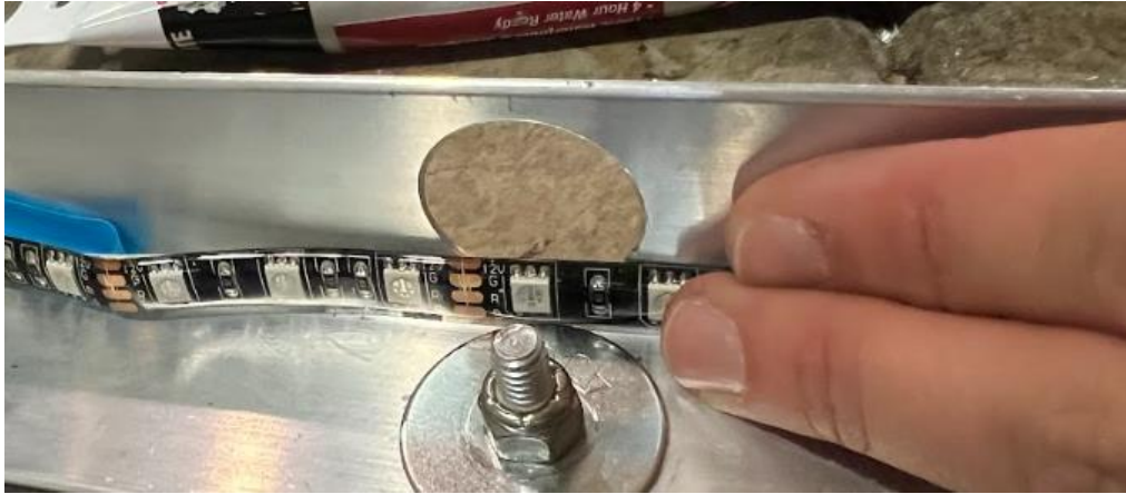
Figure 77 – Ensure the LEDs do not significantly cover the wire cutout.
