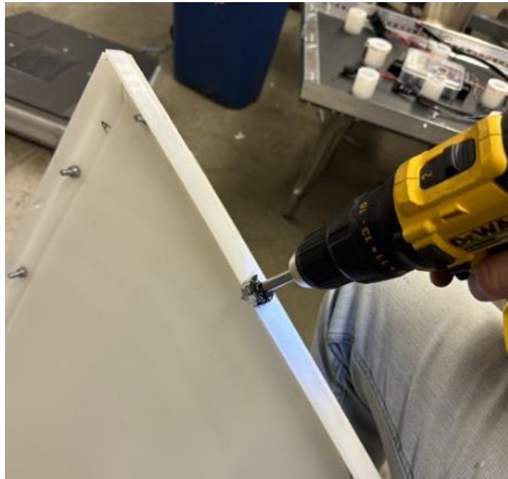
Figure 60 – Cutting the side-slot in the top angled sides using a 1" Forstner bit.
