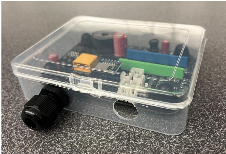
Figure 99 – Enclosure with PCB and front left gland installed.
