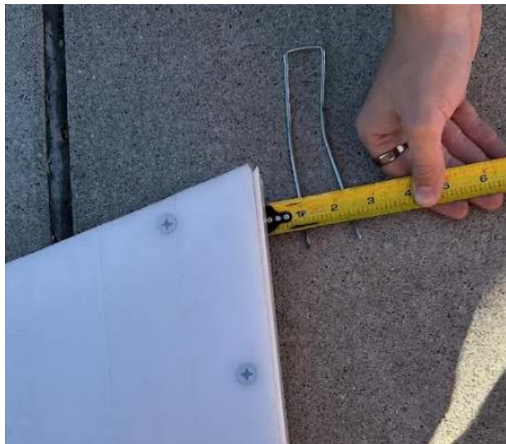
Figure 37 – Kick test result from using the tile on concrete with rubber feet. The tile moved 5/4” after 1 kick.
