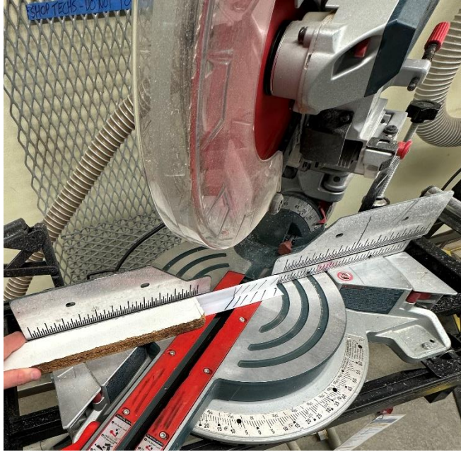
Figure 58 – 90-degree UHMW stock being cut to size using a miter saw set to a 52.5-degree angle, and scrap wood used to help hold stock against the fence.
