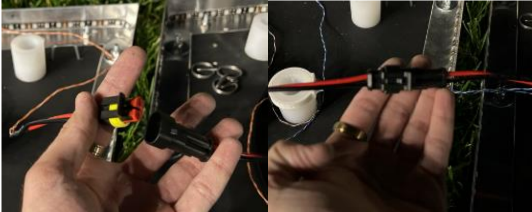
Figure 133 – Plug in Tile A's orange wire/connector to Tile B's blue wire/connector. This should occur within Tile A.
