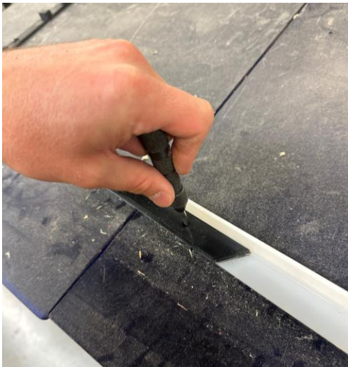
Figure 27 – Using a marking jig to center punch a hole.
