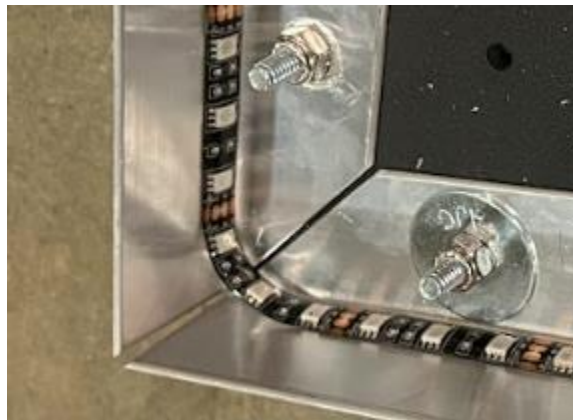
Figure 78 – Do not sharply bend the LEDs when transitioning around corners. Leave an adequate bend radius as seen above.
