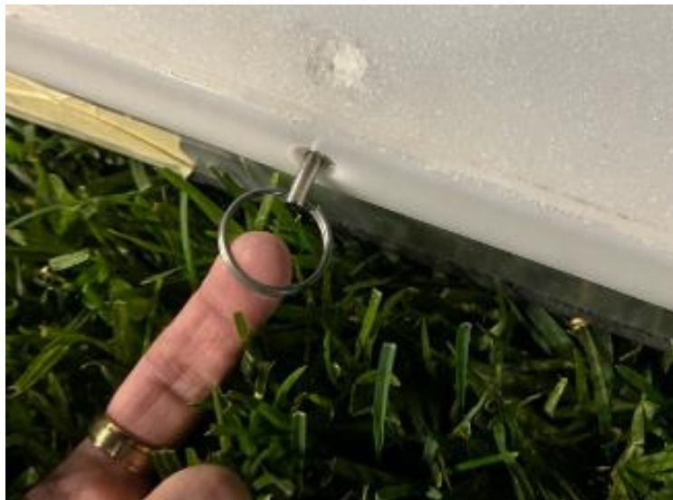
Figure 124 – Quick-release pin. Pull on the ring to remove the pin.
