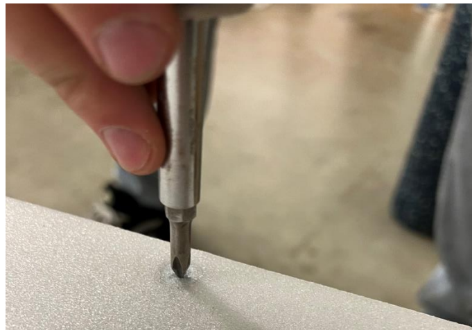
Figure 72 – Using a Philips head screwdriver to poke a hole in the grip tape.
