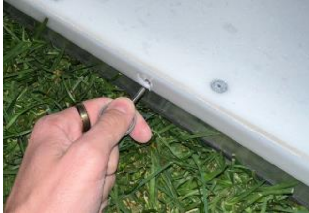
Figure 153 – Reinserting the quick-release pins. Make sure the pin goes through both the white top panel and metal hole. Ensure all 3 are replaced on every tile.
