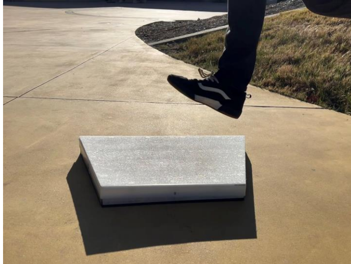
Figure 22 – Tile being administered a hefty blow from a 180 lbm participant jumping.
