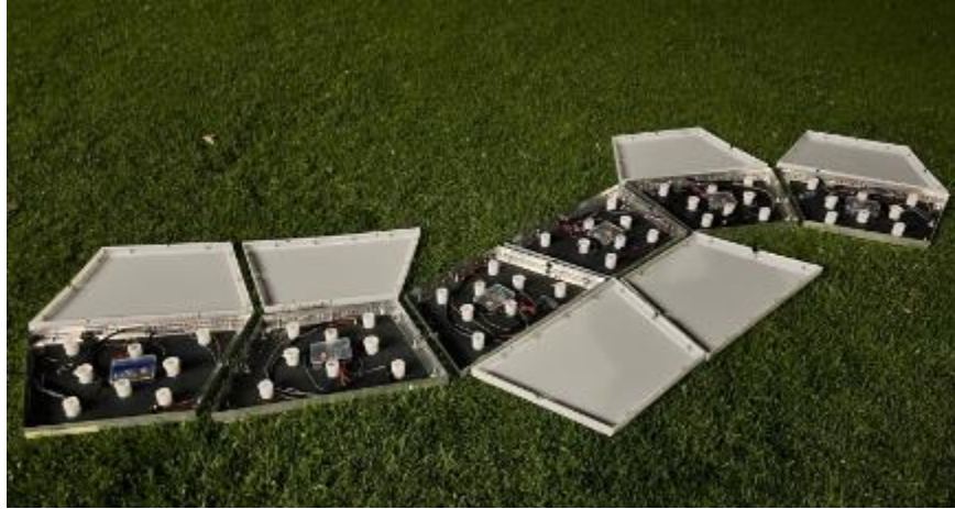
Figure 125 – Path with all lids removed. Place lids face up if the ground is dirty to avoid getting the grip tape unnecessarily dirty. Leave space next to every tile for working room.
