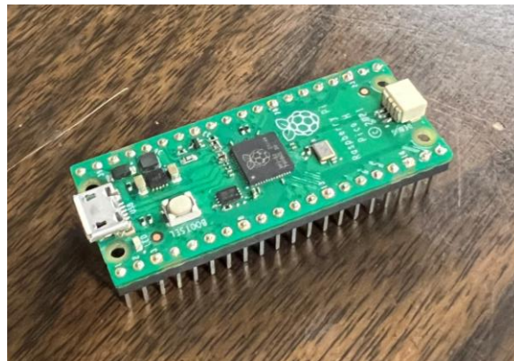
Figure 6 – Raspberry Pi Pico microcontroller board.
