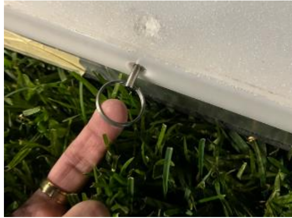
Figure 140 – Removing the quick-release pins.
