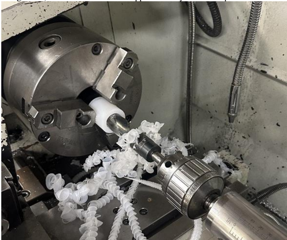
Figure 64 – Larger diameter counterbore being turned on the lathe.
