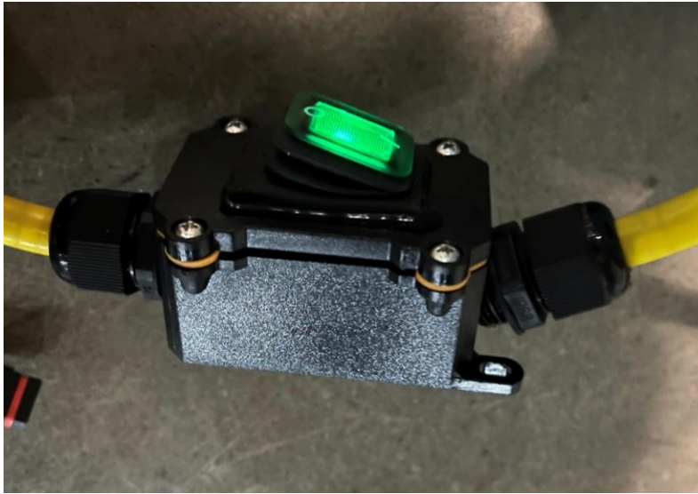
Figure 12 – On/Off power switch leading to the power supply.
