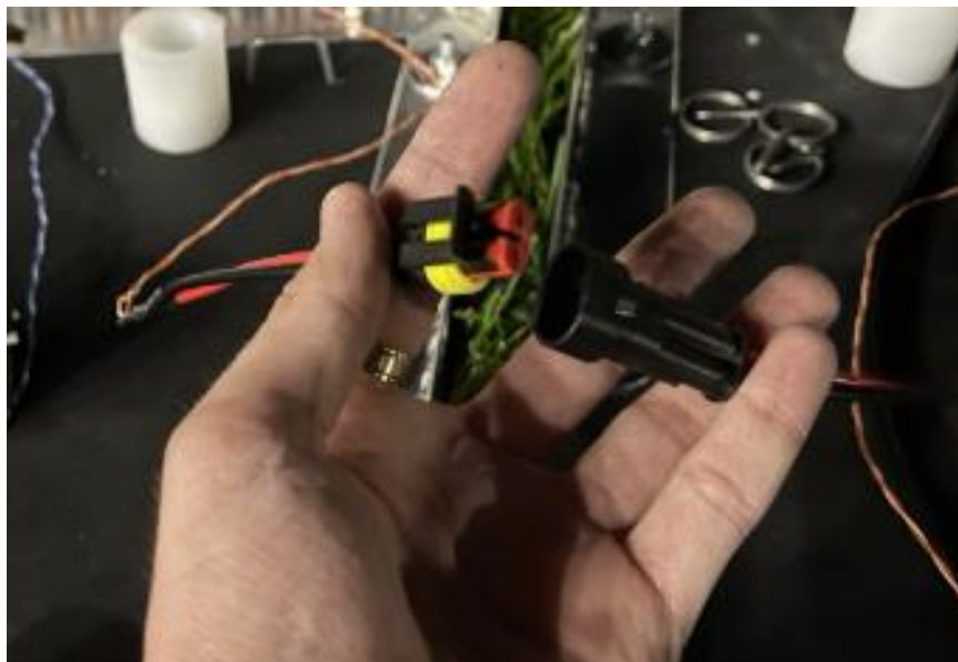
Figure 143 – Unplug orange/blue connection and feed the blue wire back through the side wire hole into its original tile.
