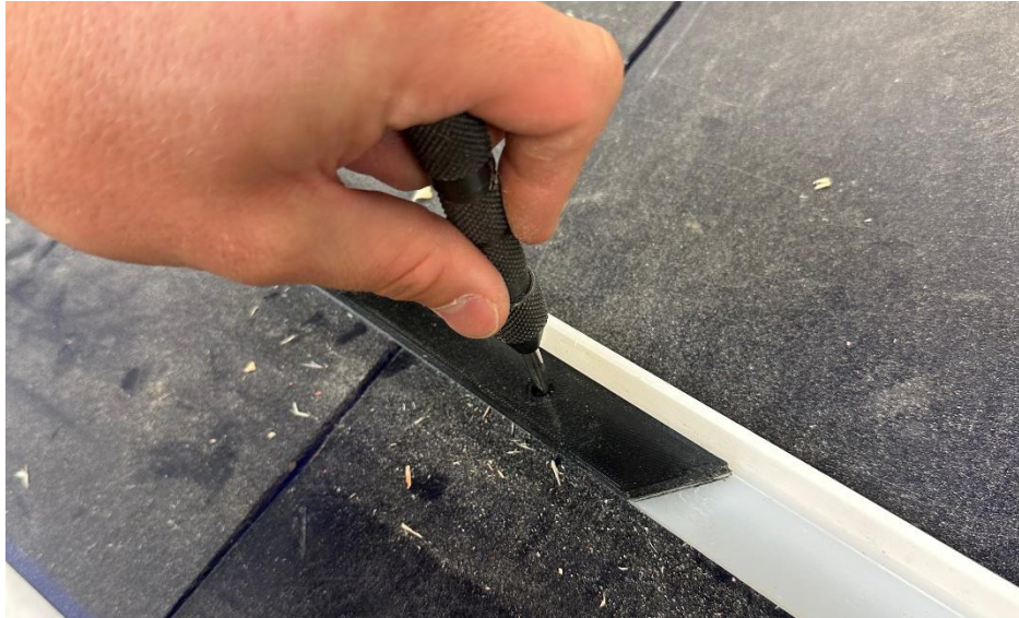
Figure 56 – Using a center punch to mark the hole locations in the stock UHMW.
