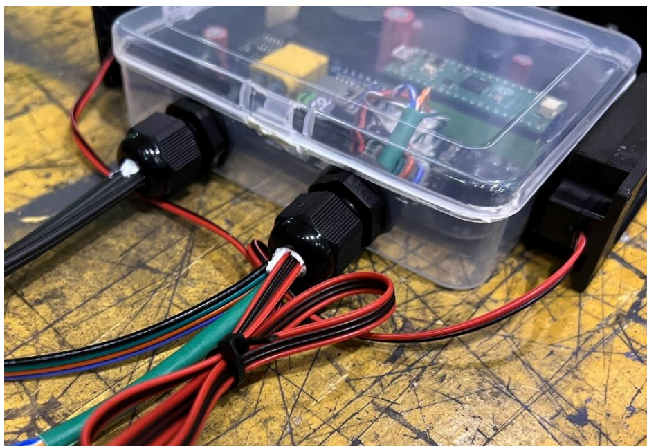
Figure 104 – Finished electronics enclosure with sealed glands.
