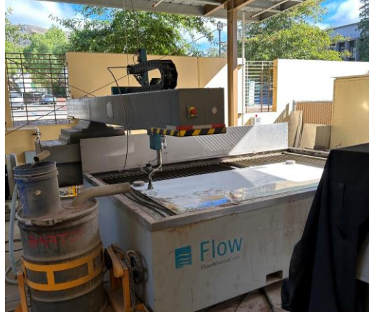
Figure 24 - Water jet cutting tiles.
