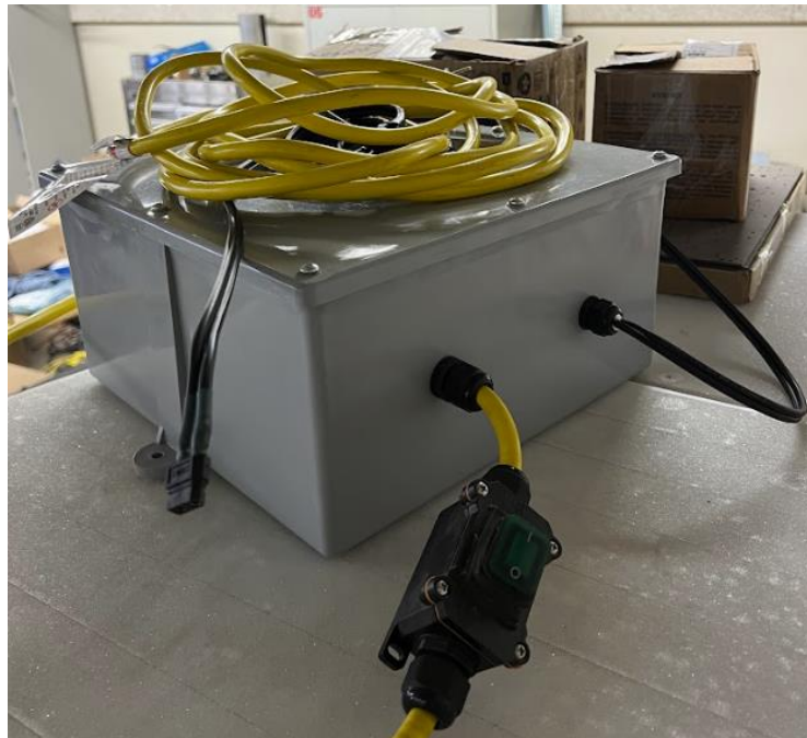
Figure 13 – Full power supply box, fitted with extension cord and the tiles' power cable.
