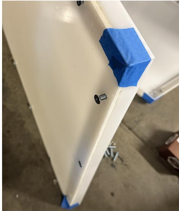
Figure 70 – Taped corners for top assembly.
