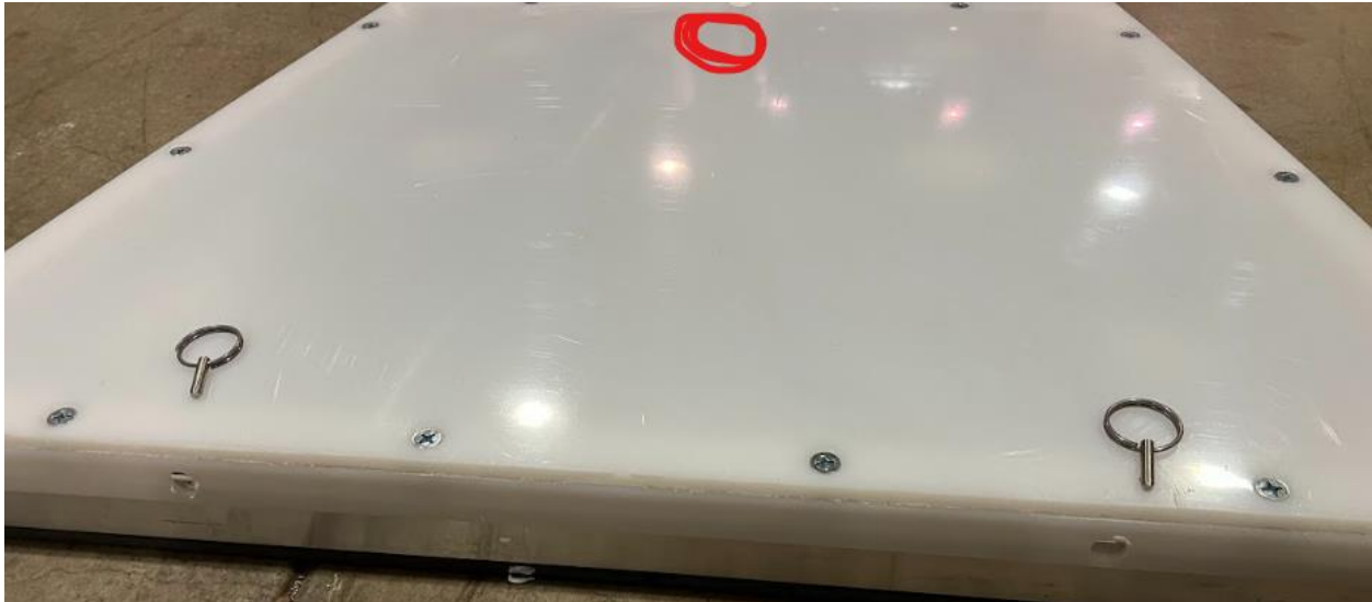
Figure 86 – Three quick-release pins should be placed in the holes under the three locations above. Note that there should be a quick-release pin in the red circle.
