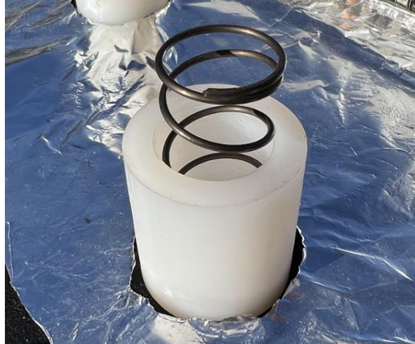
Figure 15 – Spring seated in internal support. This method proved to be quite easy and much simpler than the previous method of using bolts to do so.
