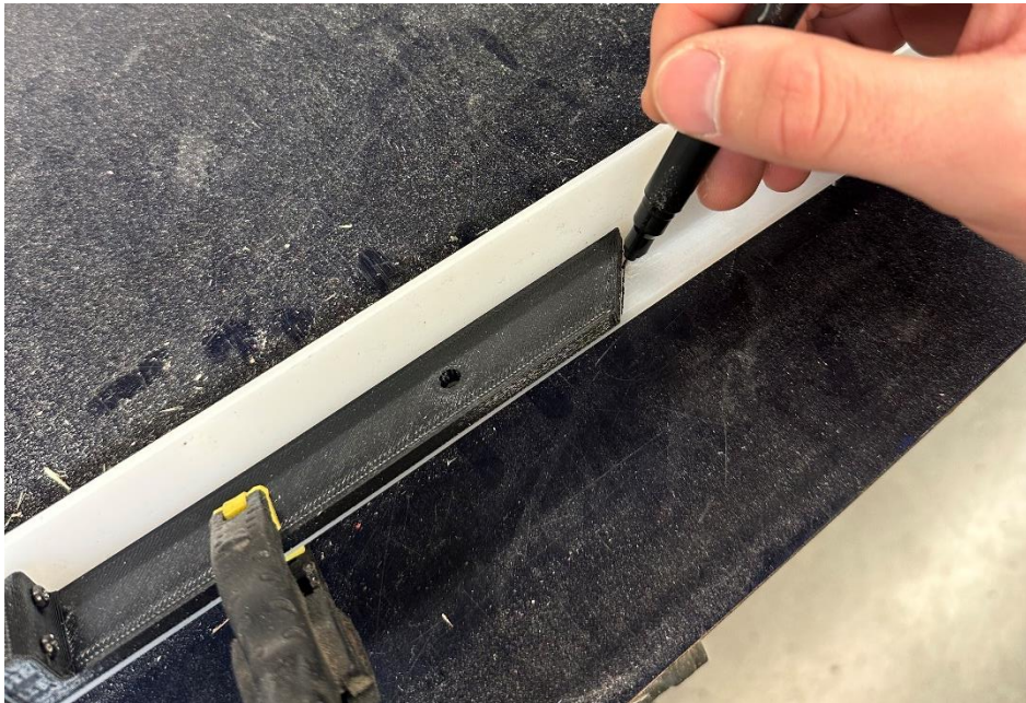
Figure 55 – Marking of UHMW stock to be cut.
