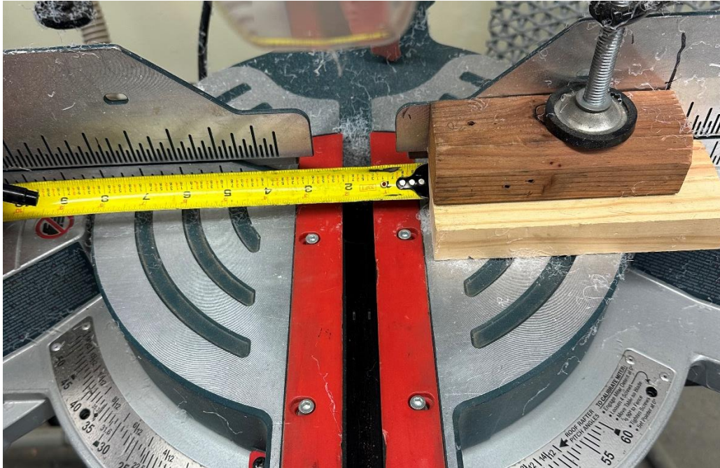
Figure 61 – Wood stop clamped down at 1 5/8" from face of the blade.
