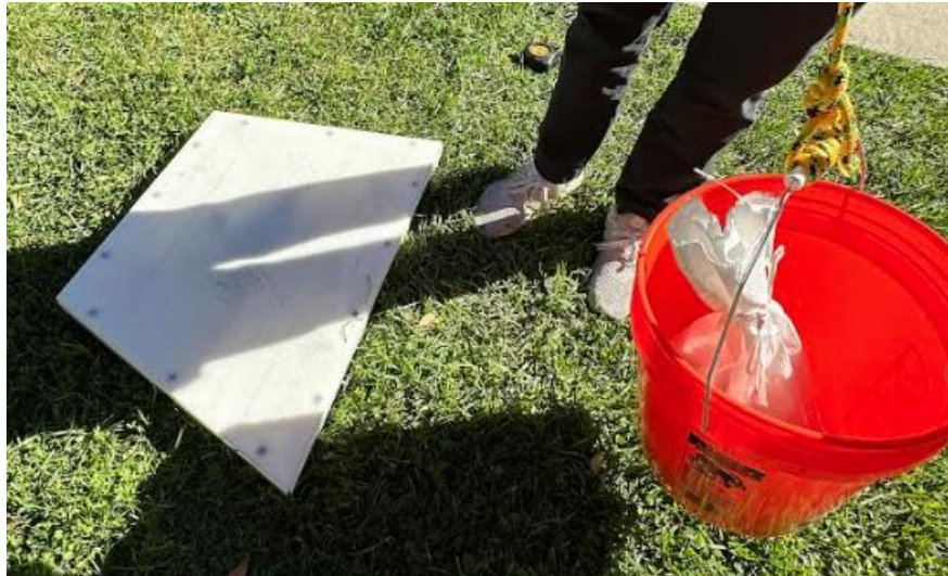
Figure 36 – Kick test setup. A weighted bucket was repeatedly swung into the side of the tile.
