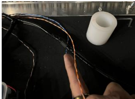
Figure 134 – Plug in Tile A's short, black power cable to Tile B's long, black power cable. This should occur within Tile A.
