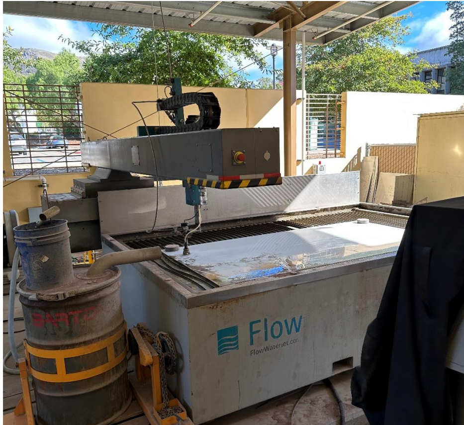
Figure 46 – Water Jet cutting top sheets from stock HDPE sheet.
