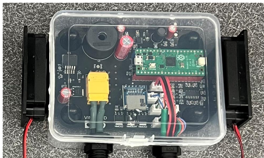
Figure 105 – Enclosure with correctly installed Pico and SD card holder.
