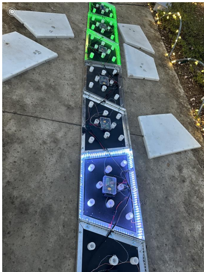
Figure 41 – Tiles experiencing the issue at the event. The start of the path is at the top of the image. Note the fully white tile.
