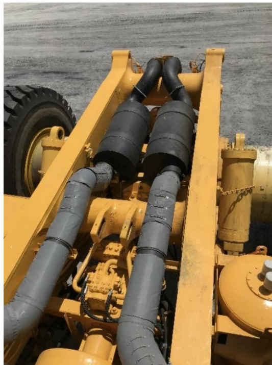
Figure 3. Minetek's Caterpillar exhaust Source: (Caterpillar Exhausts & Mufflers, n.d.)
