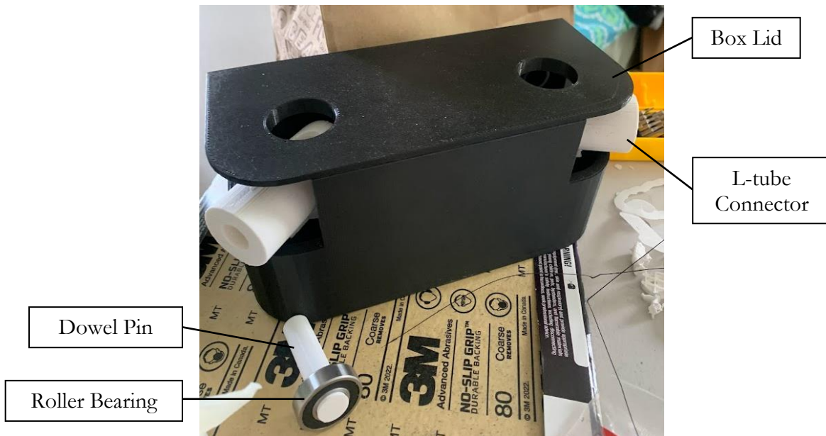
Figure 19. Motor Box with Slide-On Lid Containing Holes for Roller Bearings and Dowel Pins
