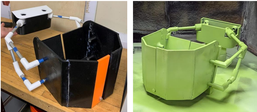
Figure 28. Scooper Assembly Before and After Spraying
