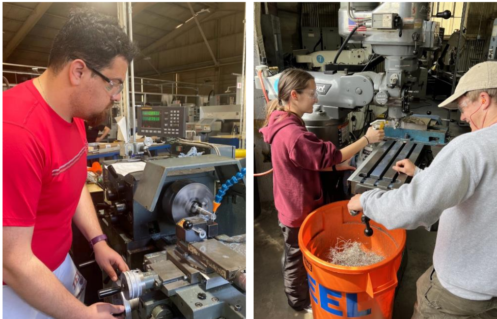
Figure 10. Turning Axle Shaft Diameters and Cutting Keyway Slots
