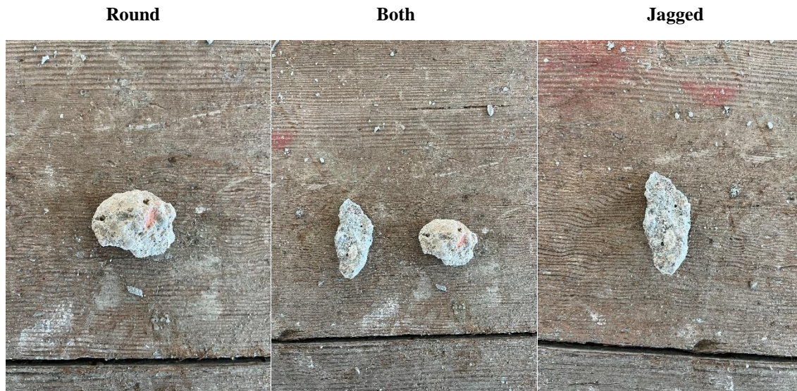
Image 1. Discrepancies of “Jagged” versus “Rounded” Recycled Concrete Aggregate.
