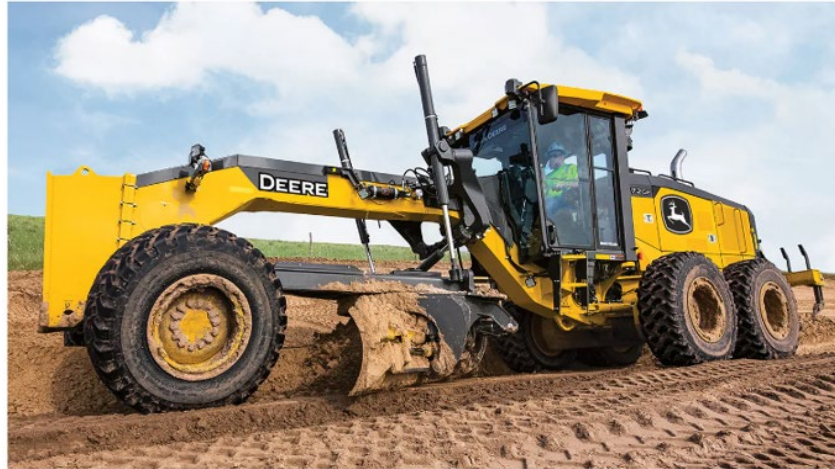
Figure 2- New SmartGrade Motor Grader, fully integrated with GPS (John Deere)
