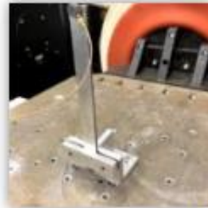
Vibration damping test to characterize the viscoelastic material's shear modulus
