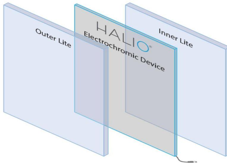
*Figure 1 – Halio Glass Product Assembly Diagram*
