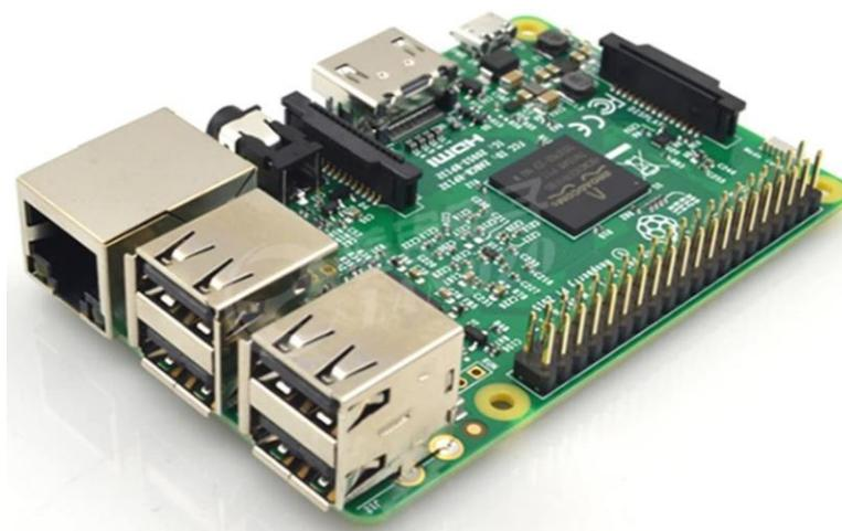
Figure10. Raspberry Pi 3 used as the microprocessor in this prototype.
