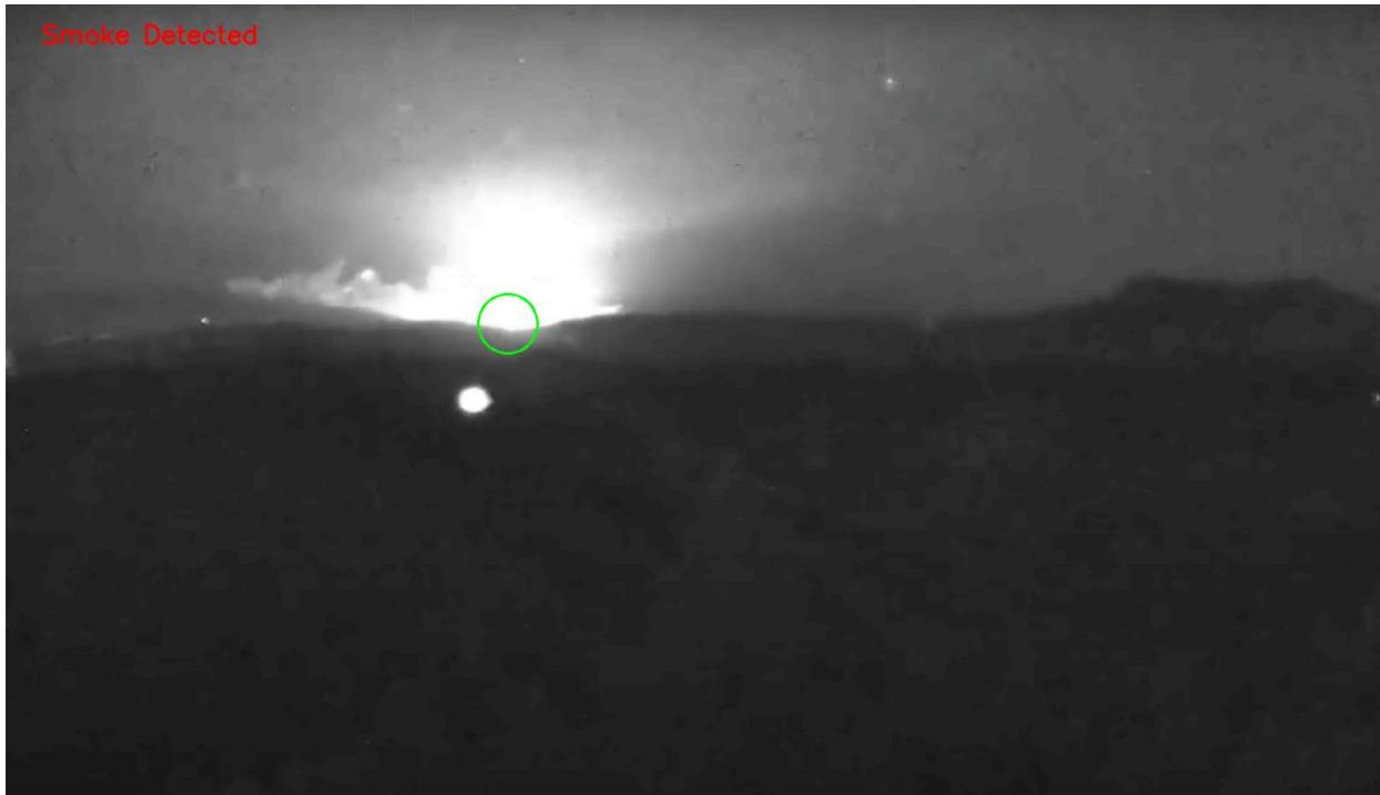
Figure 7. Annotated capture of a positive detection of smoke output by the system.
