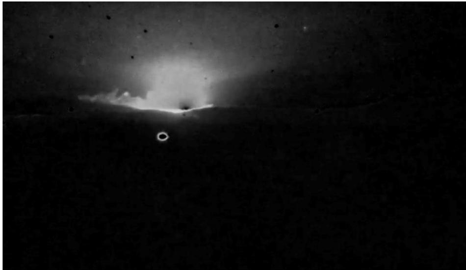
Figure 6. Resulting differenced image of the captures from the camera live feed of no smoke and with smoke.
