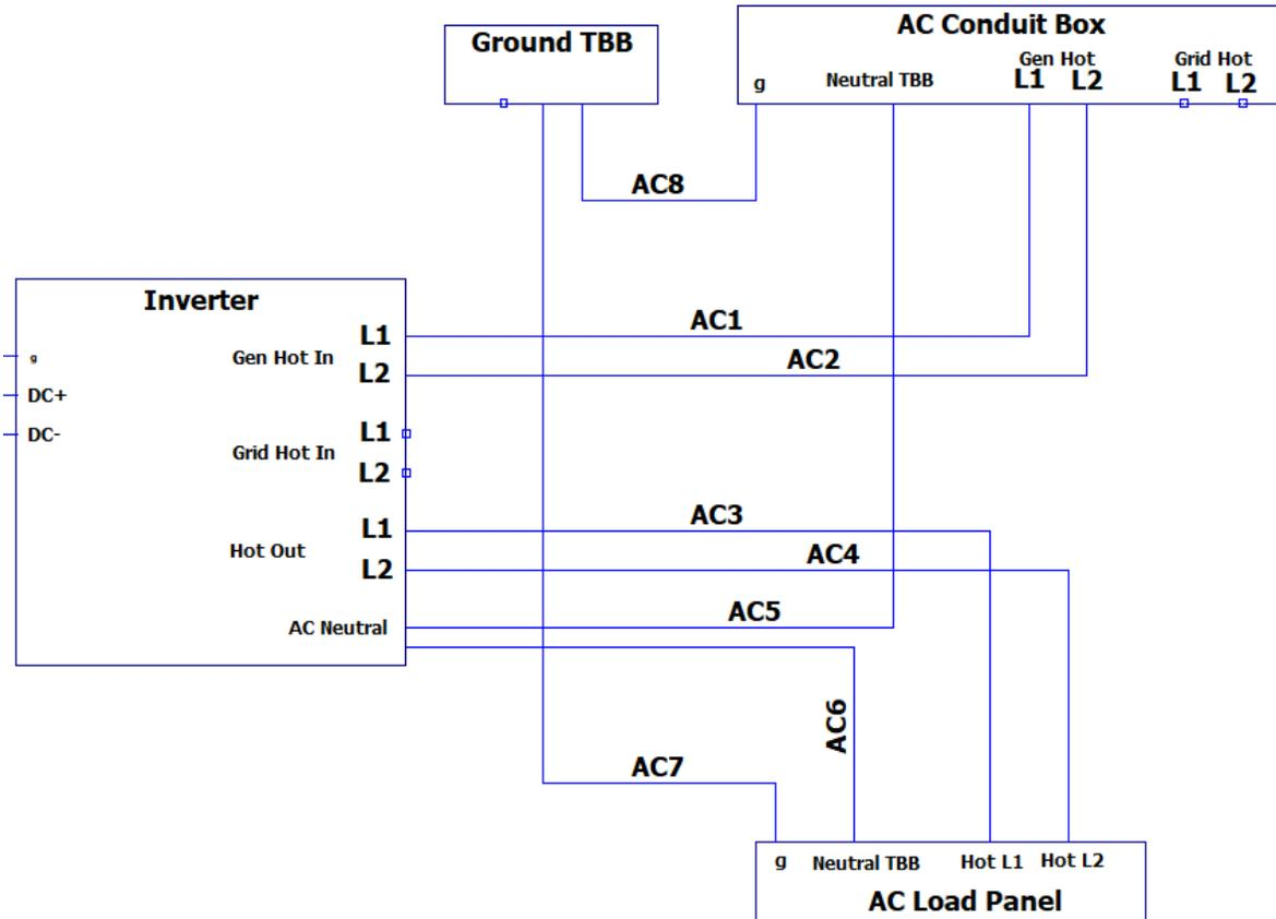
Figure 12: MST AC Wiring Diagram
