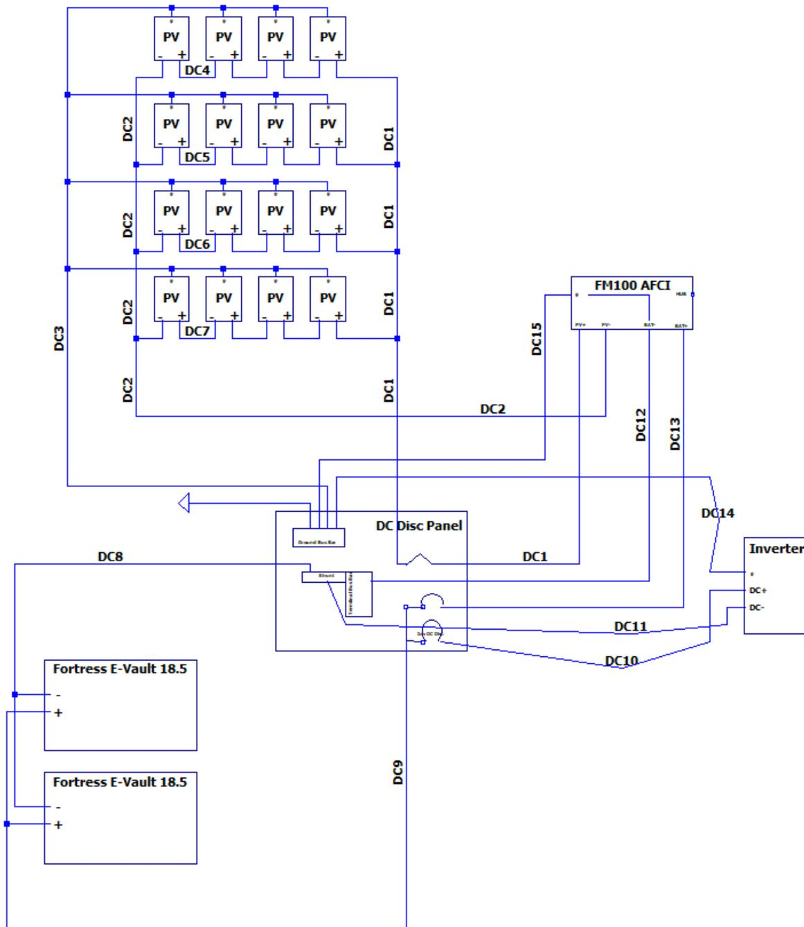
Figure 11: MST DC Wiring Diagram
