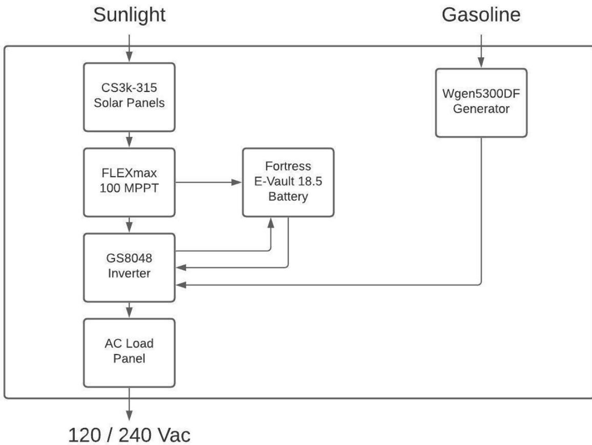
Figure 3: Level 1 Block Diagram of the MST
