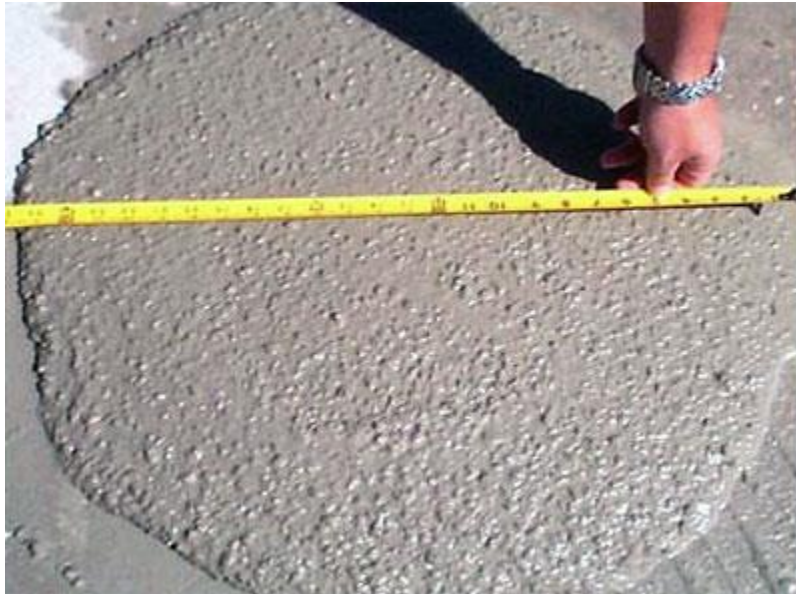
Figure 1. Slump Flow Test (Testing – Self-Consolidating Concrete)
