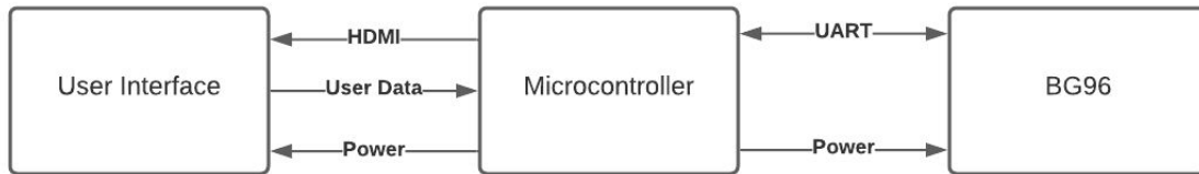
Figure3: Main Hardware Functional Blocks
