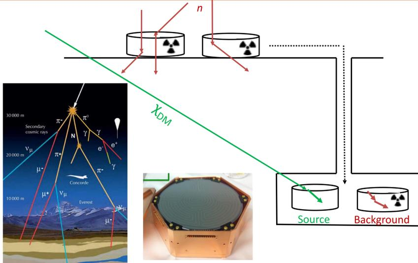
Bottom left: The germanium detectors used in the SuperCDMS detector and cosmic ray secondary showers showing multiple fundamental particles. Sources: Stanford National Accelerator Laboratory, PhysicsOpenLab.
