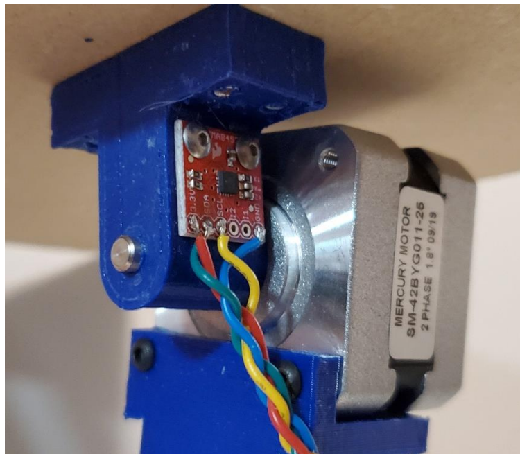
Figure 3: Accelerometer Mounting Position on Motor Output Shaft
