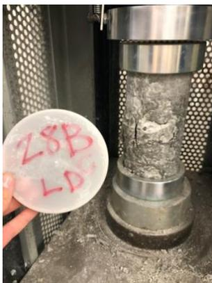
Cylinder 28B Control after strength testing
