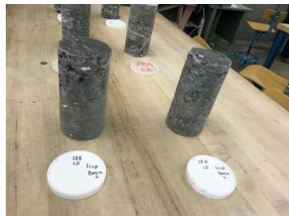
Cylinder 28A and 28B 10 oz. before strength testing
