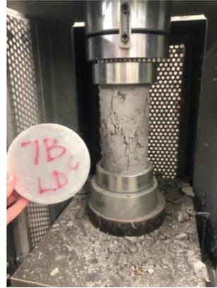
Cylinder 7B Control after strength testing
