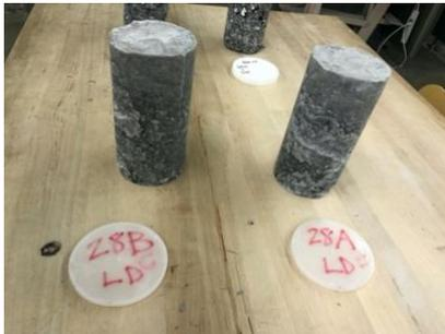
Cylinder 28A and 28B Control before strength testing
