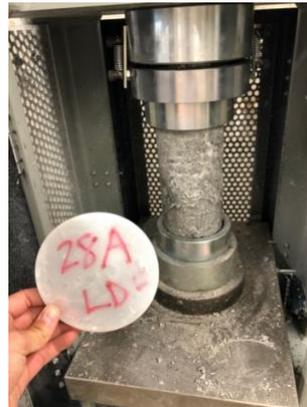
Cylinder 28A Control after strength testing
