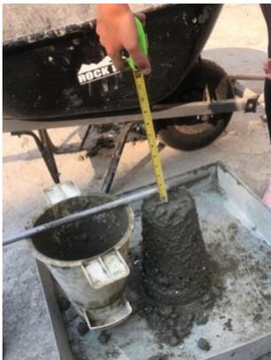
Slump test for Control batch
