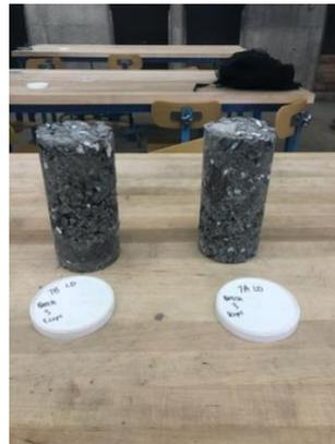
Cylinder 7A and 7B 30 oz. before strength testing
