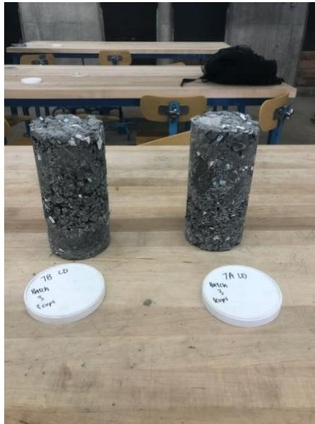
Figure 3: Cylinder 7A and 7B 30 oz before strength testing
