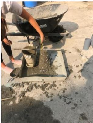
Slump test for 10 oz. face mask batch
