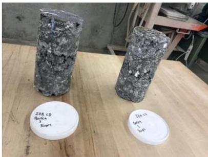
Cylinder 28A and 28B 30 oz. before strength testing
