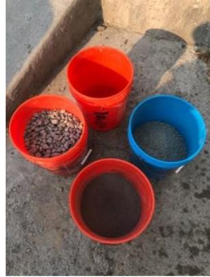
Water, coarse aggregate, fine aggregate and Portland cement
