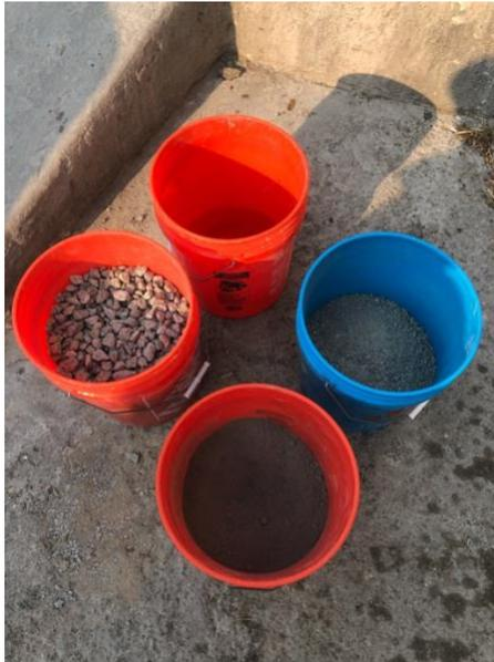
Figure 1: Aggregates, Portland cement, and water for concrete mix
