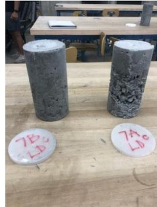
Cylinders 7A and 7B Control before strength testing
