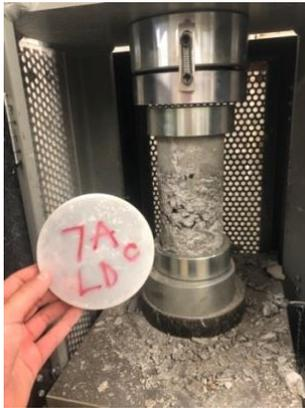
Cylinder 7A Control after strength testing
