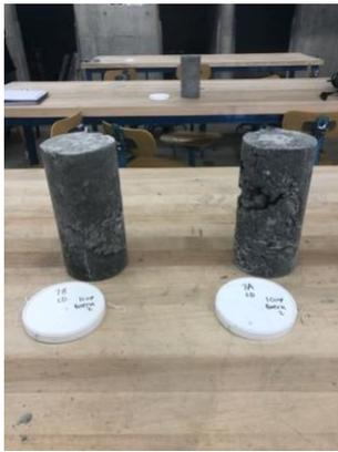
Cylinder 7A and 7B 10 oz. before strength testing
