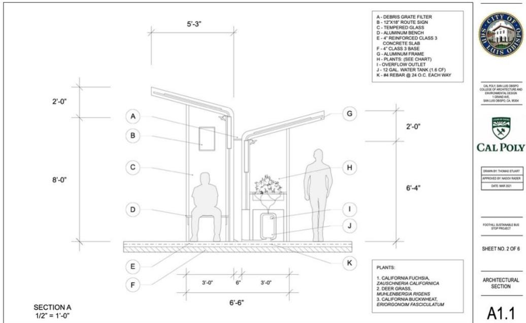
Fig. 2. Section of Architectural Plans
