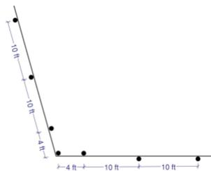
Figure 2. Post spacing and fencing placement detail
