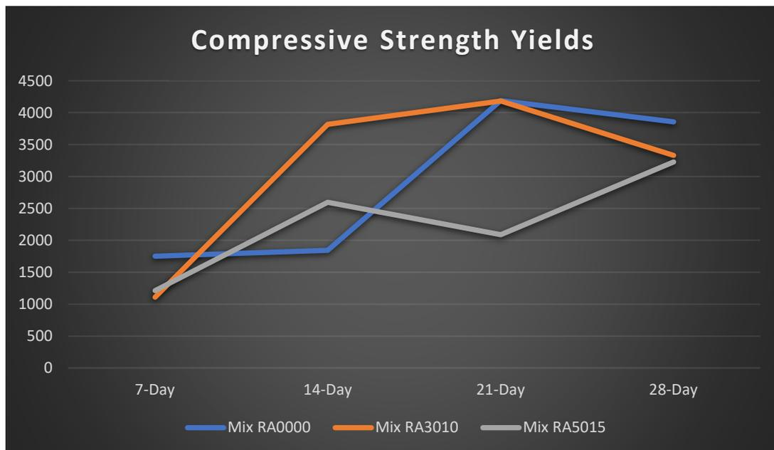
Figure 1. Compressive Strength Results per Mix
