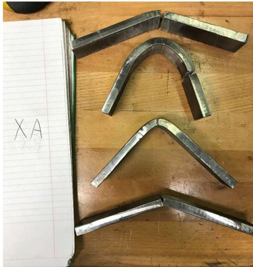
Figure 1. Profile view of procedure "XA" guided bend tests
