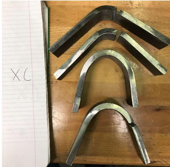
Figure 3. Profile view of procedure “XC” guided bend tests
