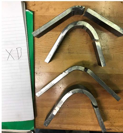
Figure 4. Profile view of procedure “XD” guided bend tests
