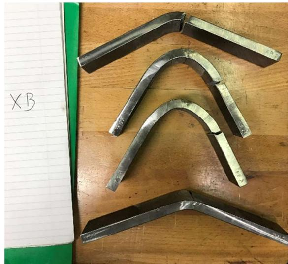
Figure 2. Profile view of procedure “XB” guided bend tests
