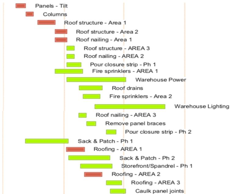
Figure 3. Project One overhead work and concrete touch up.
