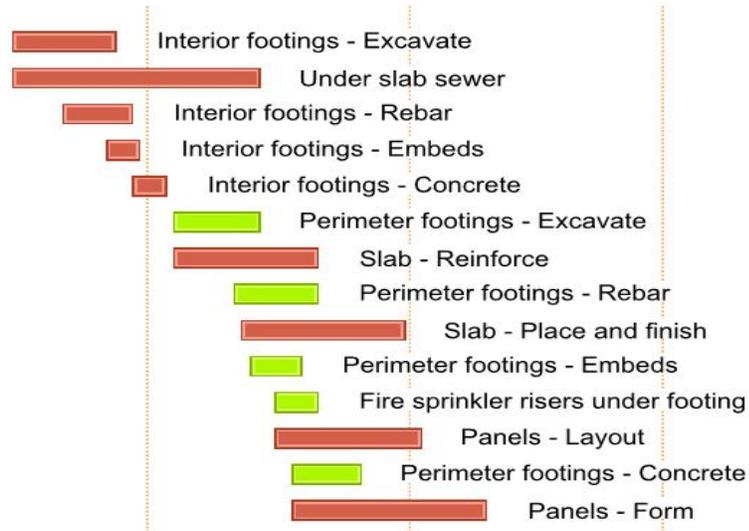
Figure 2. Project One slab, footings and panel construction
