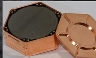
Figure 1. The SuperCDMS SNOLAB low mass dark matter detector in cryogenics system at SLAC
