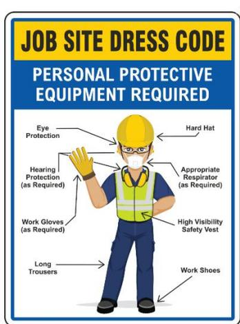
Fig 8: Sign Example of PPE for SST
